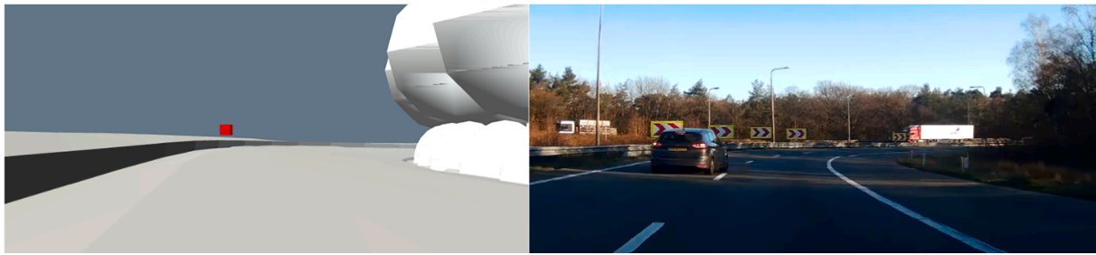
Fig. 3. On the left the analysis of “Zicht” on the visibility of the curve signs. The red object in the 3D model is the object “Zicht” checks along the alignment, in this case a curve sign, positioned above the guardrail (the dark grey line). On the right, this exact viewpoint is shown in the real life situation. (For interpretation of the references to colour in this figure legend, the reader is referred to the web version of this article.)
