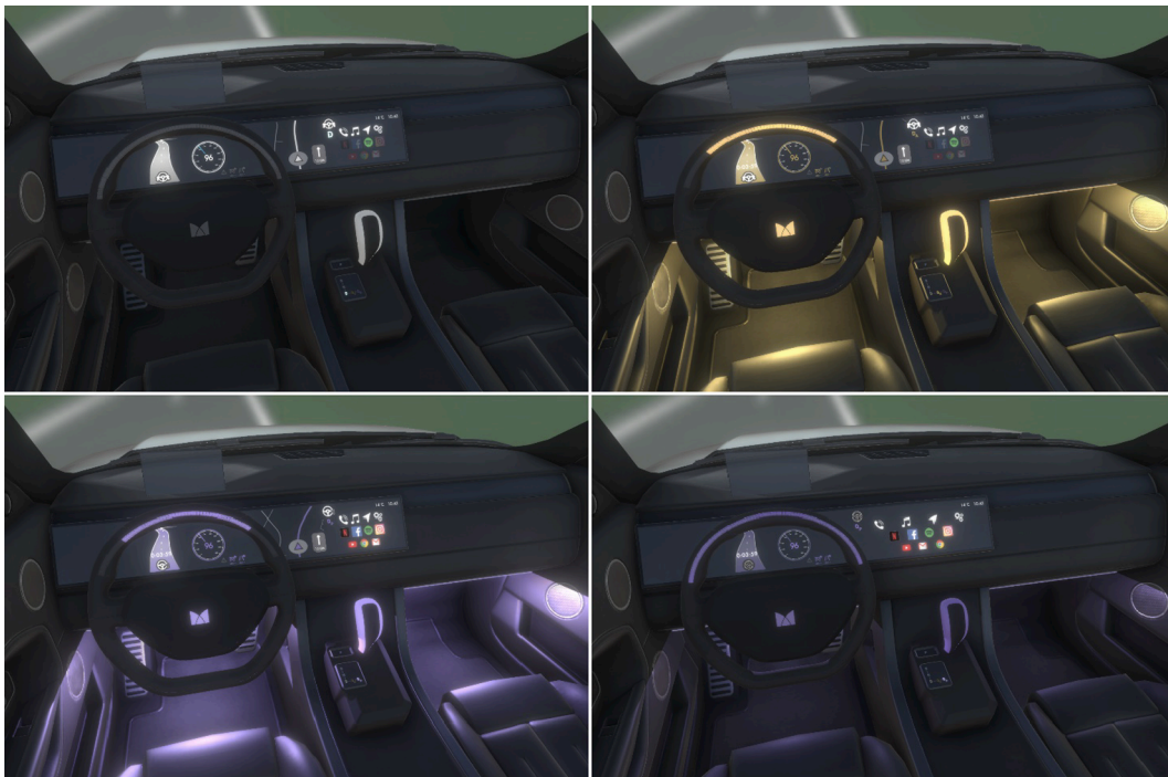
Fig. 6. The HMI design in the four different modes resulting from Phase 3 (stills from the VR environment). The design is communicating the ‘Manual’ (M) mode in the upper left picture, ‘Continuous Mediation’ (CM) in the upper right picture, ‘Standby’ (SB) in the lower left picture and ‘Time-to-Sleep’ (TtS) in the lower right picture.
