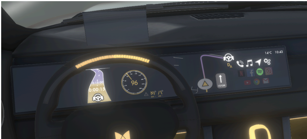
Fig. 7. The three sections (in front of driver, next to steering wheel and in line with the center console) of the HMI's display and the head-up-display (HUD) in 'Continuous Mediation' (CM) with 'Standby' (SB) becoming available in 15 s, resulting from Phase 3.
