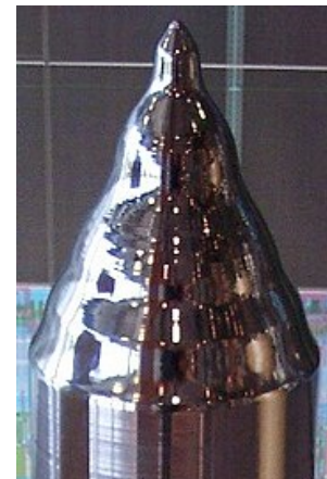
Figure 2.6: A monocrystalline silicon ingot produced by the Czochralski process [40].
