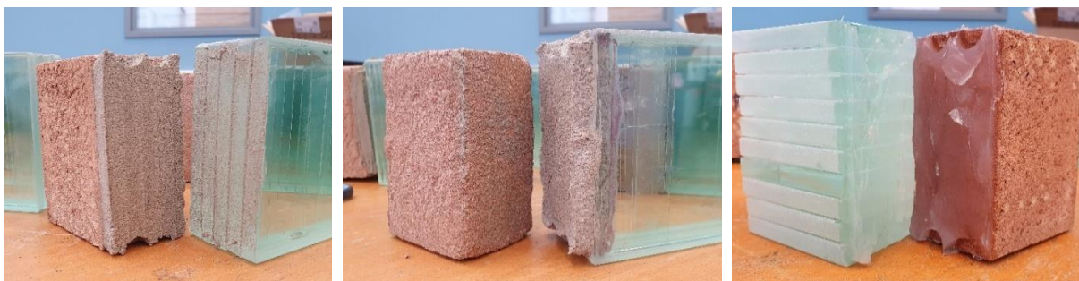
Figure 6: Left: Adhesion to glass, middle: Adhesion to brick, right: Cohesive failure
