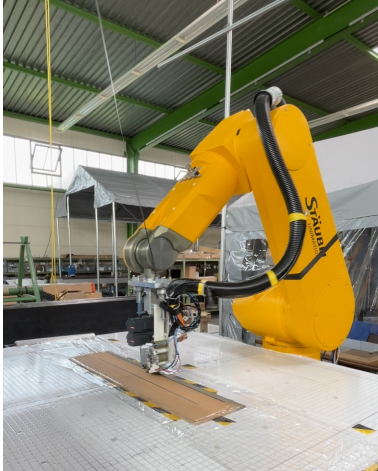
Figure 16: AFP Cell, working bed adapted with vacuum system for flat taping
