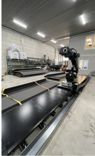
Figure 29: ABB Robot and 12-meter long track installed at 10-XL
