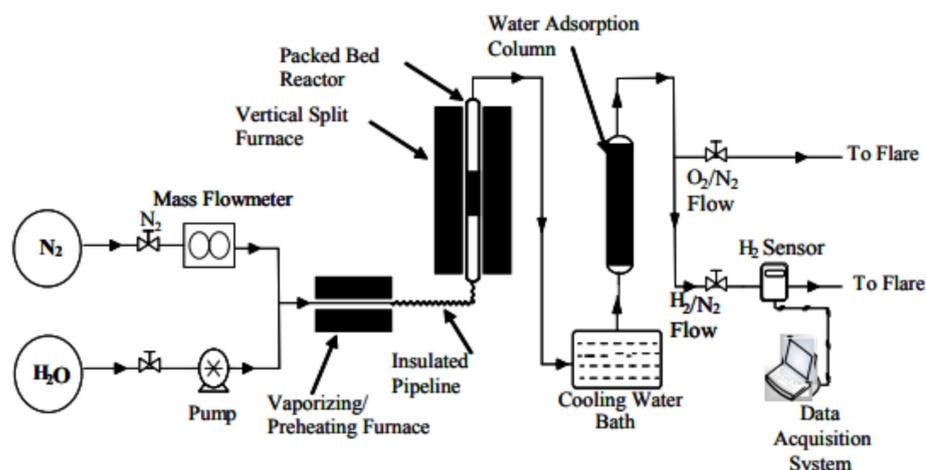
**Figure 8.** Schematic representation of the experimental setup used for thermochemical water splitting for hydrogen generation. Reprinted from [51].
