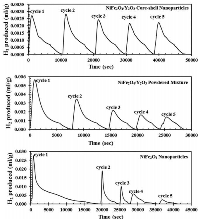
**Figure 15.** Hydrogen production rate in mL/s/g over time, showing five redox cycles for nanoparticles with a nickel ferrite core and an yttrium (III) oxide shell and a powdered mixture including nickel ferrite and yttrium (III) oxide and nickel ferrite nanoparticles. Reprinted from [103].
