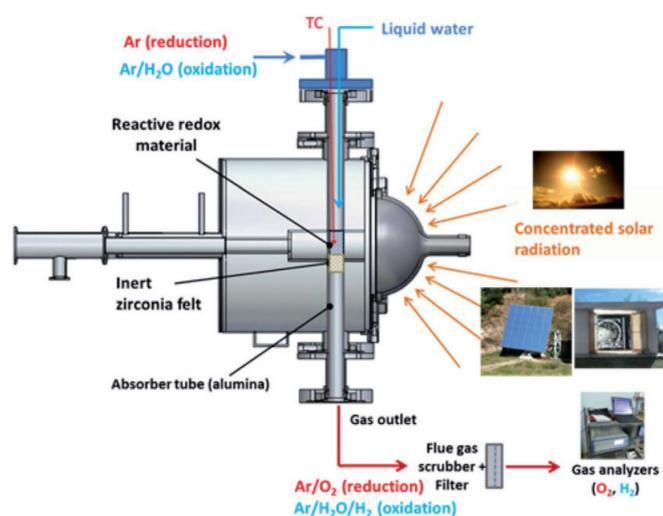
**Figure 4.** Schematic representation of a solar reactor used for thermochemical redox cycling of cork-templated ceria. The reduction temperature was  $1400\text{ }^\circ\text{C}$  and the oxidation reaction took place during free cooling when the oxygen concentration dropped to approximately zero. Reprinted from [42].
