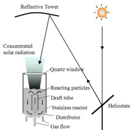
**Figure 6.** Fluidized-bed solar reactor for two-step thermochemical water splitting. The reduction reaction takes place in a nitrogen atmosphere at 1400 °C and steam is supplied for the oxidation reaction, which is conducted at 1000 °C. Reprinted from [48].
