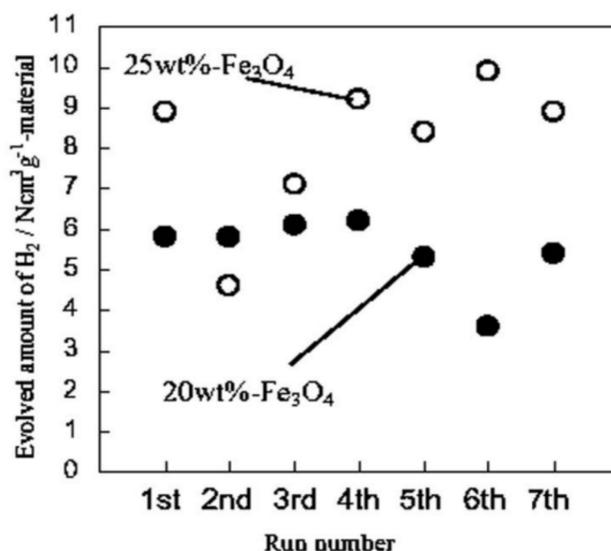
**Figure 12.** Evolved amount of hydrogen as a function of the run number for Fe<sub>3</sub>O<sub>4</sub> supported on yttrium-stabilized zirconia. The reduction temperature was 1400 °C. The solid circles represent 20 wt%-Fe<sub>3</sub>O<sub>4</sub> and the open circles represent 25 wt%-Fe<sub>3</sub>O<sub>4</sub>. Reprinted from [30].
