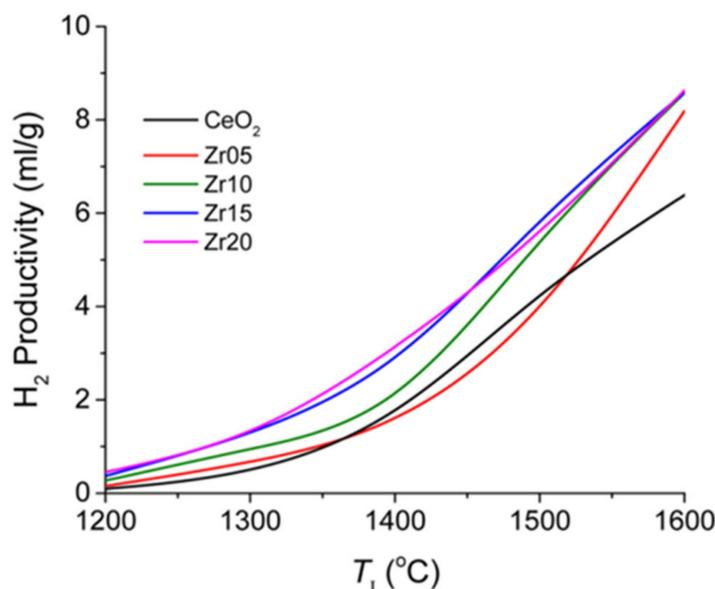
**Figure 11.** Hydrogen yields for isothermal two-step thermochemical water splitting at different doping concentrations of zirconium in cerium oxide, including cerium (IV) oxide without doping. Reprinted from [85].
