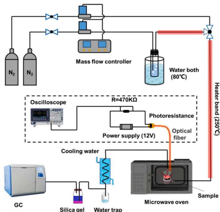
**Figure 9.** Schematic representation for performing the thermochemical water splitting cycle using  $(\text{FeMgCoNi})\text{O}_x$  supported on silicon carbide foam using a microwave oven. Reprinted from [55].
