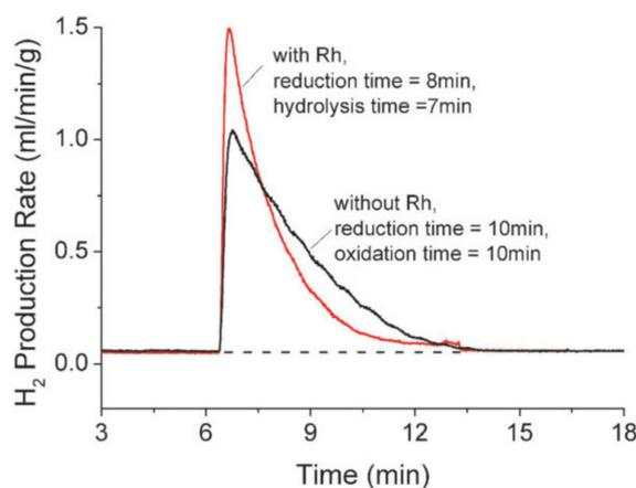
**Figure 14.** Effects of rhodium added to cerium (IV) oxide on the reduction and oxidation times, as well as on the hydrogen production rate during isothermal cycling at a temperature of  $1500 \text{ }^\circ\text{C}$ . Reprinted from [64].
