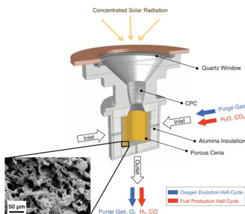
**Figure 2.** Schematic representation of the solar reactor used for thermochemical water splitting. The redox material used in porous ceria. As the same setup was used in another experiment for syngas production, carbon dioxide and carbon monoxide are also denoted in the figure, as well as a scanning electron microscope image of ceria after 23 cycles. Reprinted from [44].
