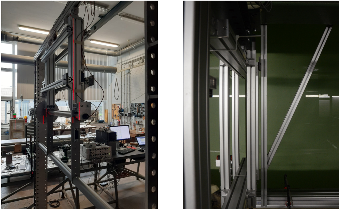
Figure A.10: The pendulum is orientated vertical when it is unloaded (left). This check is done using a laser with an included spirit level. The pendulum is perpendicular to the towing tank (right). This orientation is examined using a large L-square, made of aluminium profiles, which is aligned with the rails of the towing tank.
