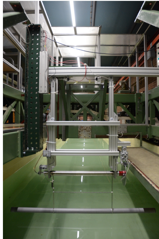
Figure A.3: Picture of the medium pendulum. In this arrangement, the length of the top part of the pendulum is 0.95 m, and the length of the bottom part is 0.4 m.
