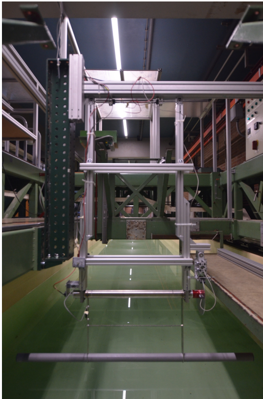
Figure A.2: Picture of the long pendulum. In this arrangement, the length of the top part of the pendulum is 1.25 m, and the length of the bottom part is 0.4 m.
