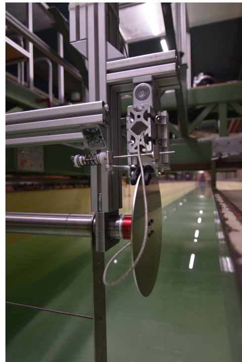
Figure A.9: Close up of the friction mechanism. In the friction mechanism, a hinge is incorporated to adjust for possible small horizontal deviations of the disc.
