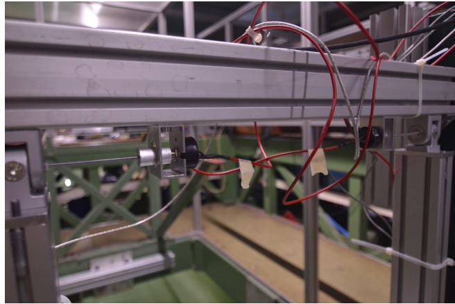
Figure A.7: Potentiometers 1 and 2 are connected to the top hinges in order to measure the angle of the top part of the pendulum.
