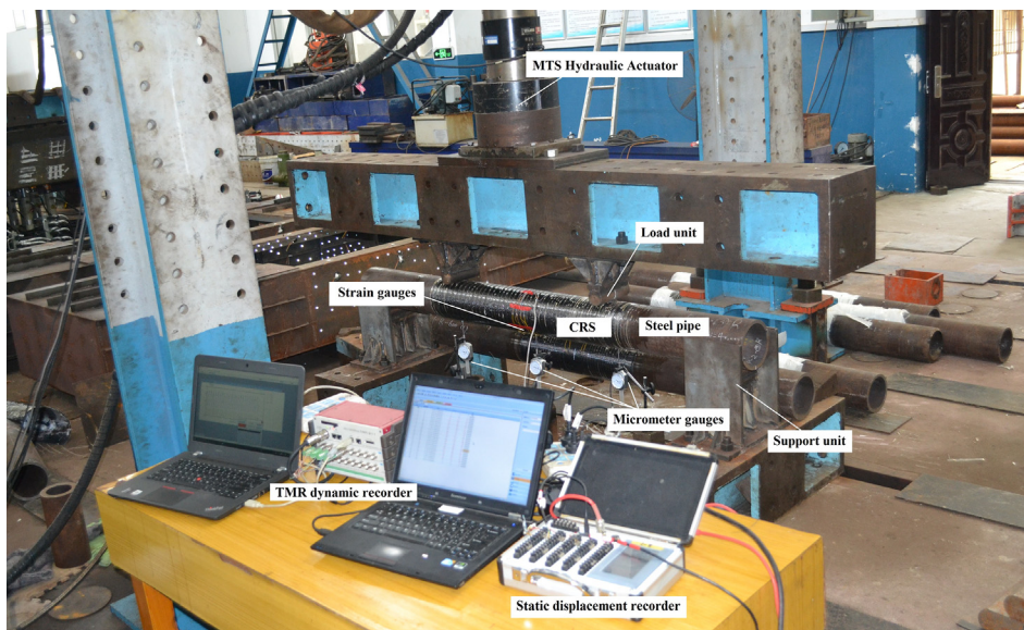
Fig. 6. Specimen and instruments installation.
