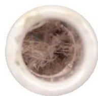
Figure 13 Deteriorated PDMS pervaporation membrane
