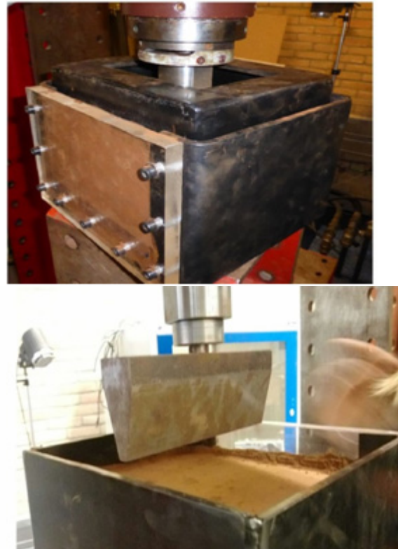
Figure 6. Consolidating the iron ore sample: top) consolidating iron ore with the top plate, bottom) starting point of the penetration phase
