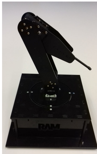
Fig. 11 Robot arm used for learning the IK model. The robot was designed and built by the Robotics and Mechatronics group, University of Twente, the Netherlands
