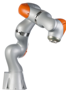
Figure 4-1: KUKA LBR iiwa robot manipulator (Image: KUKA)
