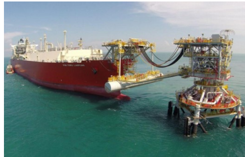
Figure 4.3: Yoke Mooring System
