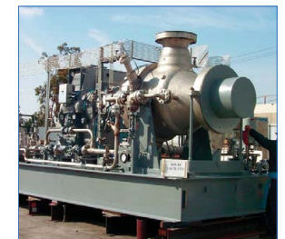
Rotoflow turboexpander-generators are packaged complete and ready for installation.
