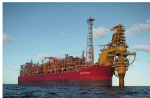
Figure 4.4: Riser Turret Mooring (RTM) System
