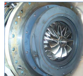
Vertically split casings ensure easier installation and assembly at the job site.
