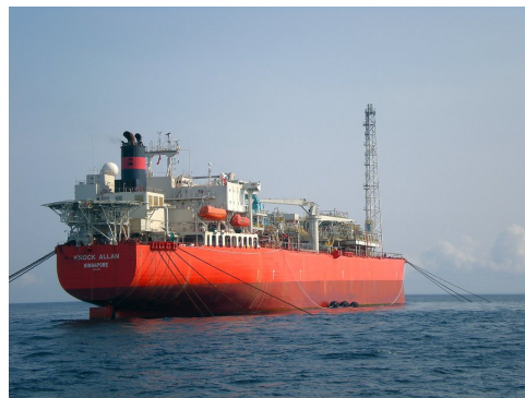
Figure 4.7: Spread Mooring (SM) System
