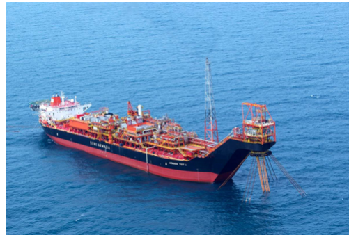
Figure 4.6: External Turret (ET) Mooring System
