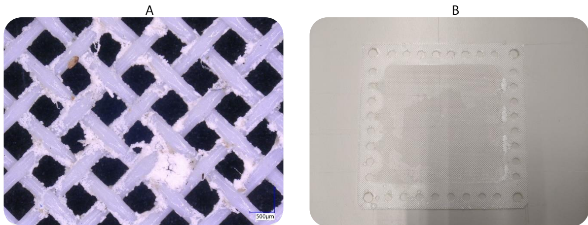
Figure 7-7 - The accumulation of, mostly Mg-based, precipitated minerals in the concentrate spacers in the ED membrane stack (A) after the treatment of multiple batches of real SDRW. The white precipitates especially accumulated at the entrance (at the right) of the spacer (B).
