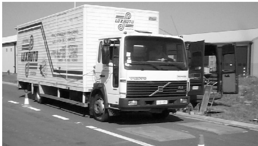
Figure 156. The Volvo FL6 truck in front of the artificial road unevenness installed at the test site (Degrande & Lombaert, 2002)
