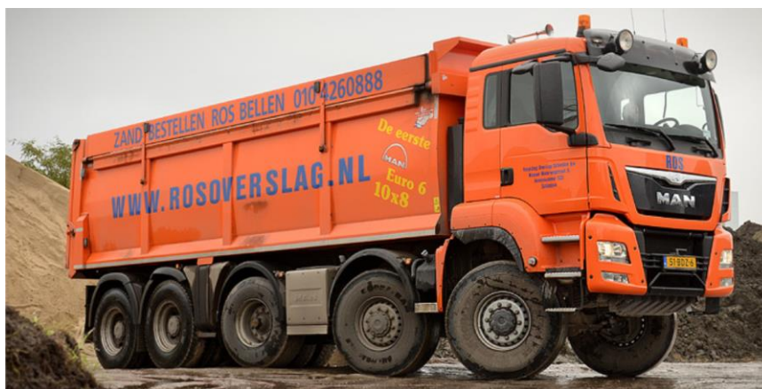
Figure 174. MAN TGS 10x8 WSA sandtruck used for the measurements at the VU Amsterdam site (modderaandebanden.nl, 2019)
