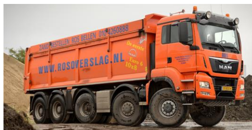
Figure 6o. MAN TGS 10x8 WSA sandtruck used for the measurements at the VU Amsterdam site (modderaandebanden.nl, 2019)
