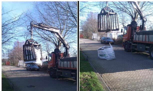
Figure 4. Execution of experiment for determining transfer function of vibrations from soil to floor: a falling Bigbag at a certain distance from the building (Eilders, 2015)
