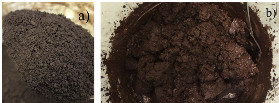
Fig. 13. Forming large agglomerates after adding 4% extra moisture content; a) MC_{as,rec} , b) MC_{as,rec+4\%} .
