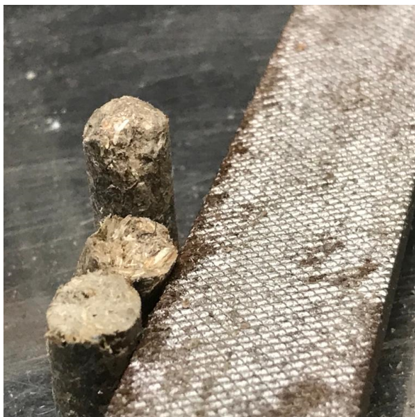
Figure 3.3: Pellets with their convex and concave ends, and one filed flat
