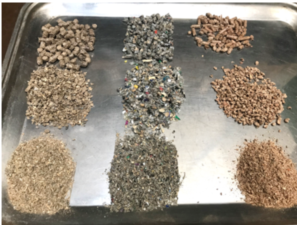
Figure 1.2: From Left to Right: Waste Wood, RDF, Fresh Wood From Top to Bottom: Pellets, Lumps, Fines
