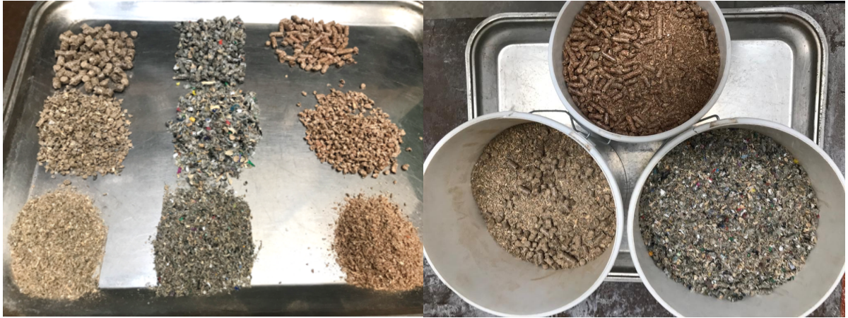
Figure 3.16: From Left to Right: Waste Wood, RDF, Fresh Wood Figure 3.17: Waste Wood, Fresh Wood and RDF Pellets at 30% From Top to Bottom: Pellets, Lumps, Fines
