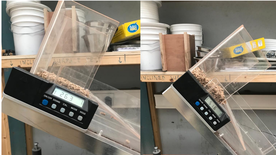
Figure 3.10: Angle of tilt test device. Left no flow, right flow
