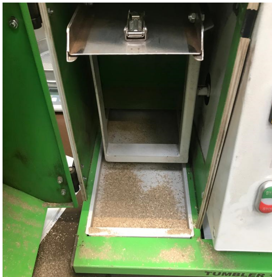
Figure 3.2: Tumbler 1000+ produced by Institut fuer Bioenergie with fines created by testing waste wood pellets
