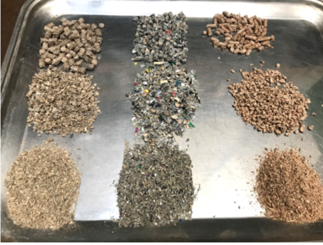
Fig. 1: From Left to Right: Waste Wood, RDF, Fresh Wood From Top to Bottom: Pellets, Lumps, Fines
