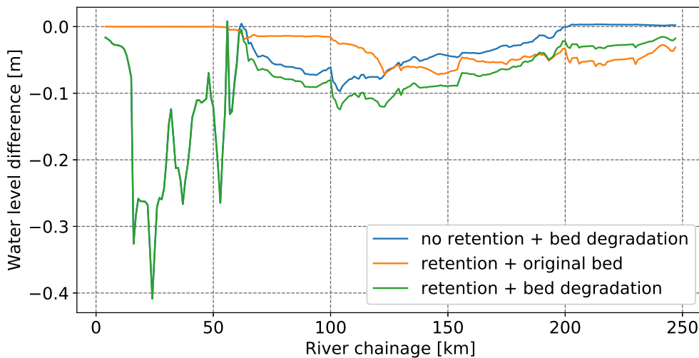
Fig. 5.1.: Maximum water level differences for a 3950 \text{ m}^3/\text{s} ( T = 3000 year) discharge wave for model runs with and without active retention areas for the original and degraded bed levels. The water levels are plotted relative to the water levels resulting from a model run with original bed levels and no active retention areas.
