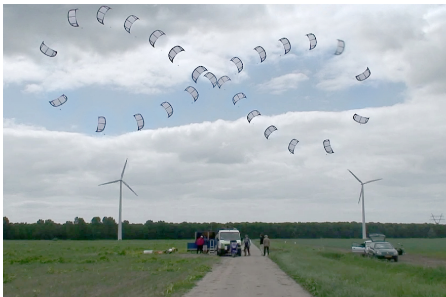
Figure 2. Composite photo of a crosswind figure-of-eight maneuver ( \Delta t = 1 s) of a tube kite with 25 \text{ m}^2 wing surface area [9].
