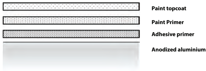
Figure 6.21 Schematic representation of chromic acid anodized aluminium with the adhesive primer and paint layers (not to scale).
