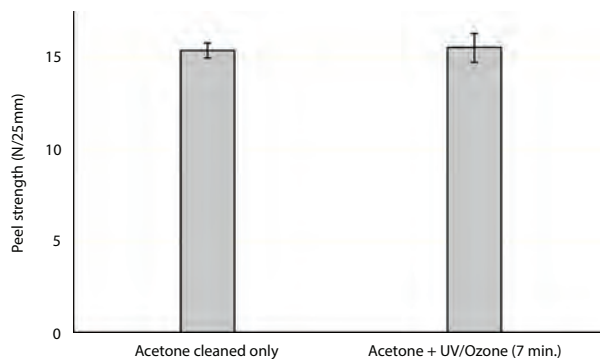
Figure 6.20 Floating roller peel test results for acetone cleaned only and those with a 7 minutes added UV/Ozone treatment of CFRP to CFRP bonded samples.
