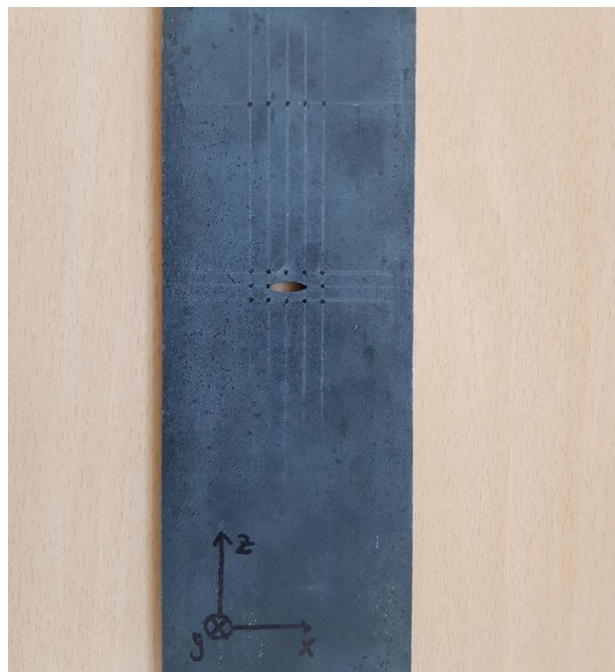
Fig. 6 Test specimen with extra row of five measurement points 50 mm above elliptical hole.
