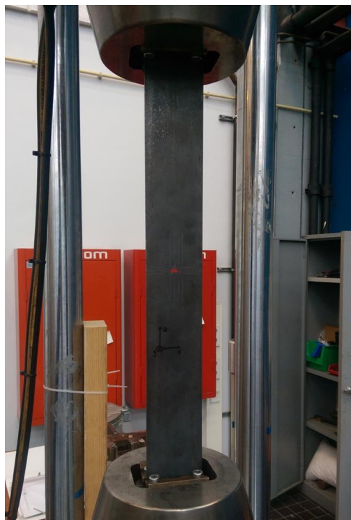
Fig. 2 Specimen while clamped in the MTS fatigue testing machine.
