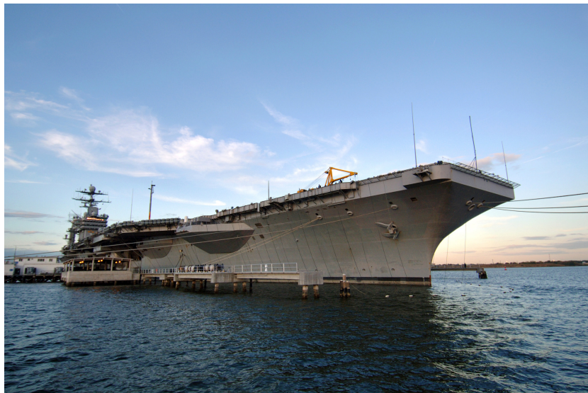
Figure 1.1: USS Harry S. Truman (CVN 75), a United States Navy aircraft carrier, being depermed at the Lambert's Point Deperming Station in Virginia. Note the electrical cables looping around the hull. (Source: https://commons.wikimedia.org/wiki/File:US_Navy_051115-N-2984R-123_The_Nimitz-class_aircraft_carrier_USS_Harry_S._Truman_(CVN_75)_undergoes_a_deperming_evolution_at_the_Lambert%27s_Point_Deperming_Station_in_Norfolk,_Va.jpg , Public Domain.)
