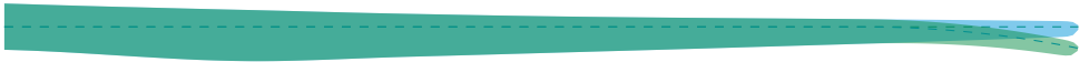
Figure 8.4: Schematic representation of a wind turbine blade with a swept tip defined by z_{start}/R = 0.8 and y_{tip}/R = -0.02 , blade planform based on the IEA 15 MW reference wind turbine [15]
