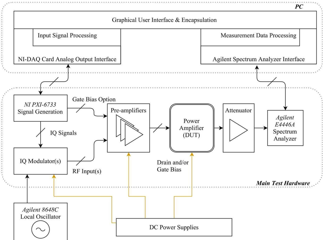
Figure 3.2: A schematical decomposition of the power amplifier test system.
