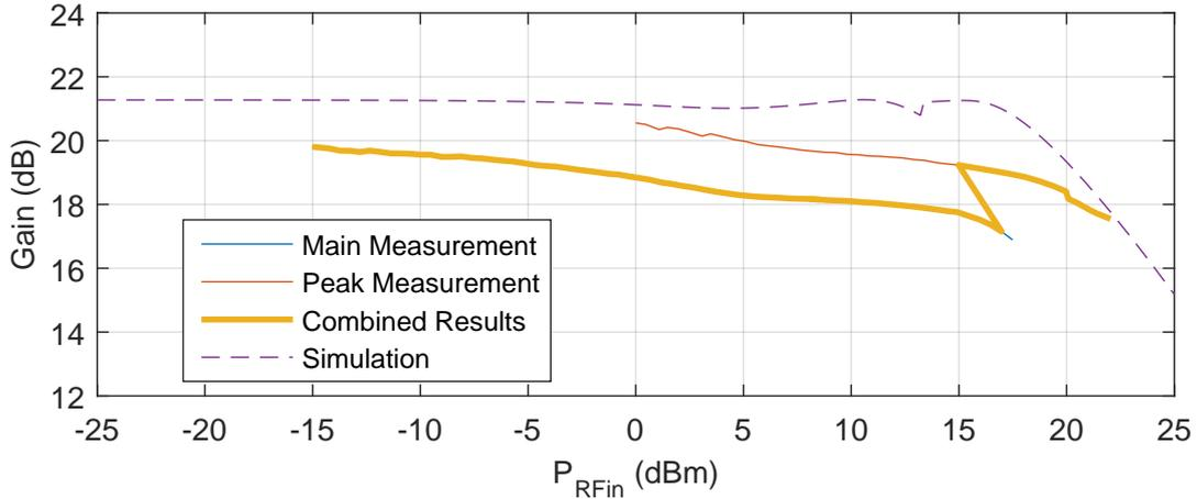
Figure 9.4: Comparison of gain measurement and simulation for a varying bias interpolating supply PA biased at 28 V peak transistor drain voltage.
