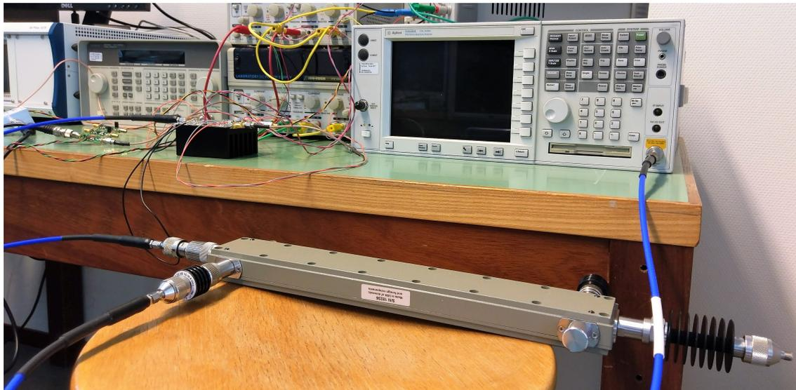
Figure 7.2: Spectrum analyzer and the coupler connected to each other to prevent high power inputs to the spectrum analyzer.
