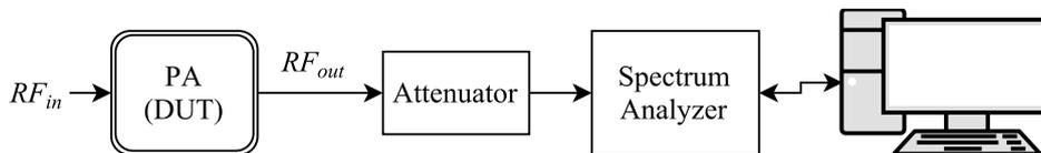
Figure 7.1: Simplified overview of the spectrum analyzer subsystem.
