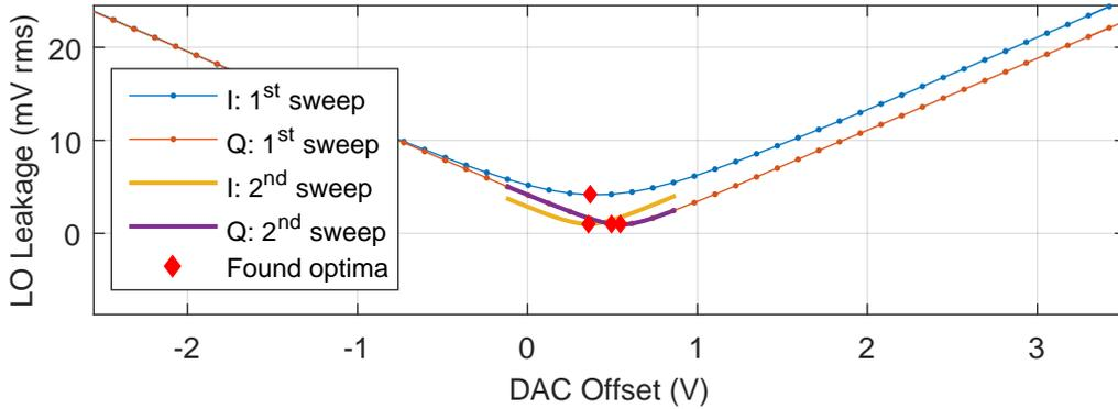
Figure 5.4: Calibration results for DC offset. This calibration performed four sweeps in total: I followed by Q and both repeated once, as described in Section 5.2.3.
