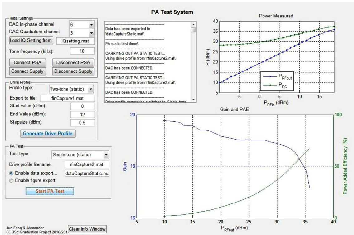
Figure 8.2: PA test system GUI after having performed a gain and efficiency measurement using a single tone.
