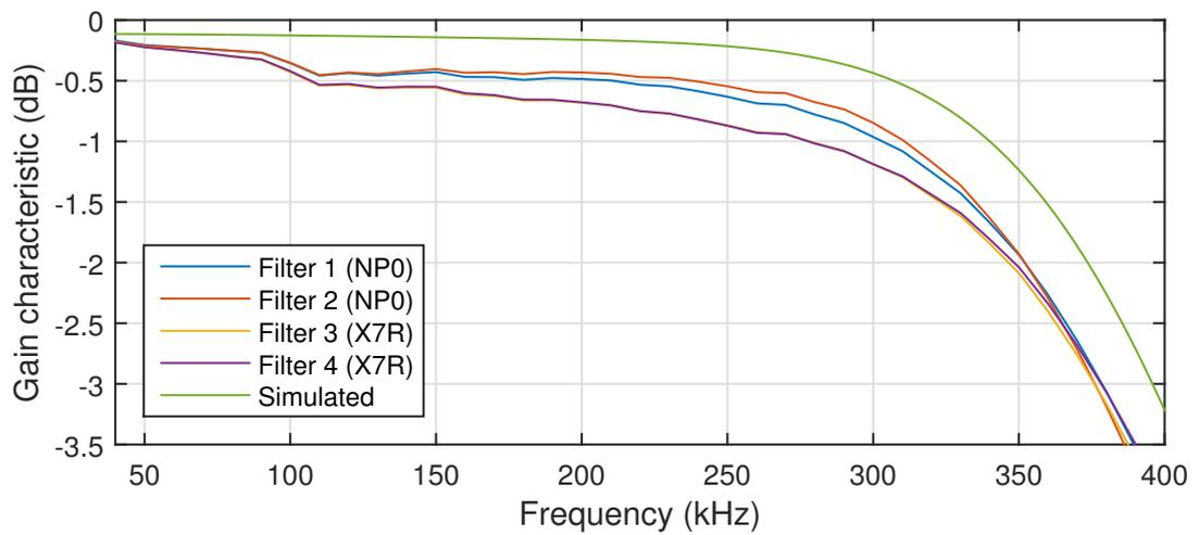
Figure 4.8: Gain characteristic of the four produced LC-filters, with the filters labeled in order of production, and of the simulated filter
