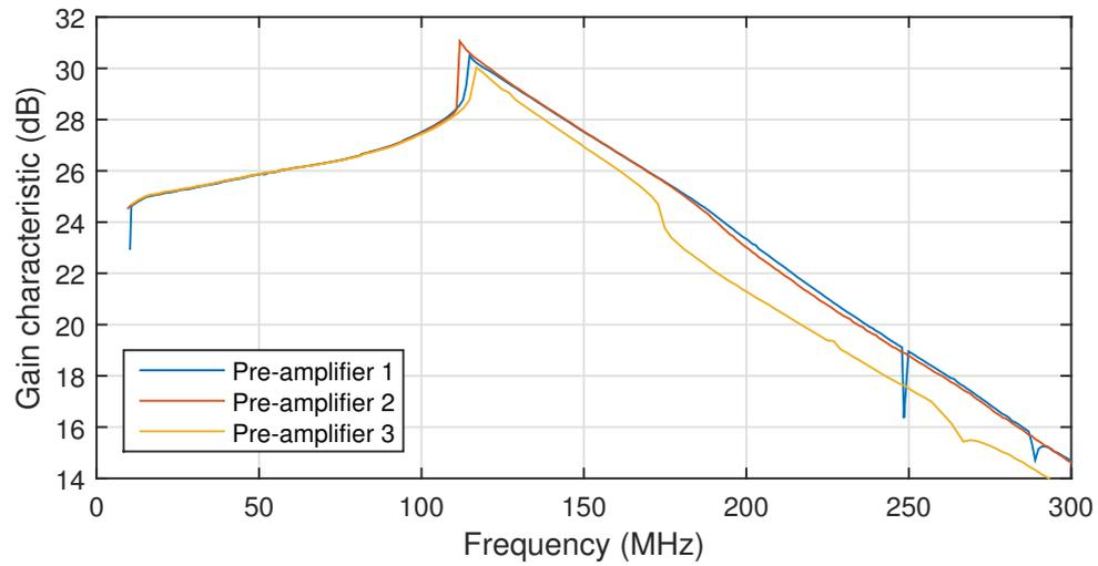
Figure 6.5: Gain over frequency of the pre-amplifiers with a -8 dBm input.
