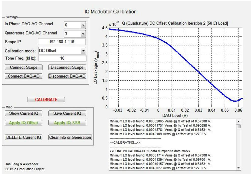
Figure 5.5: Screenshot of the GUI used for IQ calibration.
