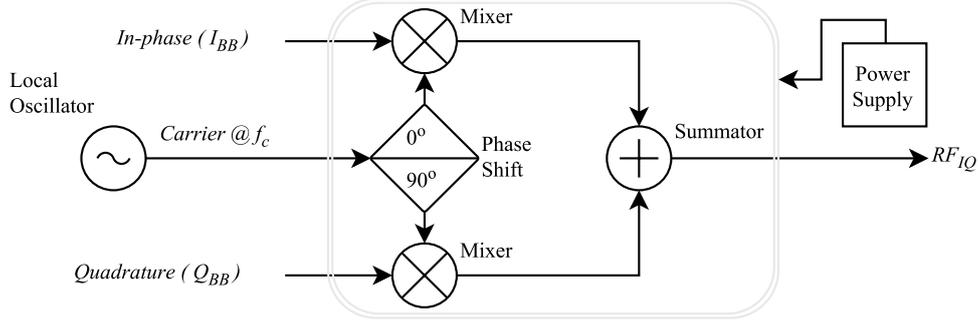
Figure 5.2: Operation of an ideal IQ modulator.
