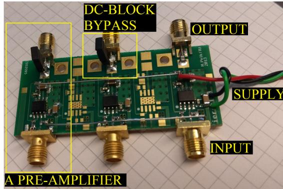
Figure 6.4: Pre-amplifier board including the DC-block bypass pins for 2 of the amplifiers.
