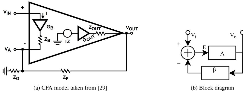
Figure 6.2: Simple models for noninverting amplifiers with negative feedback. (a) Simplified current feedback amplifier. (b) Negative feedback block diagram.
