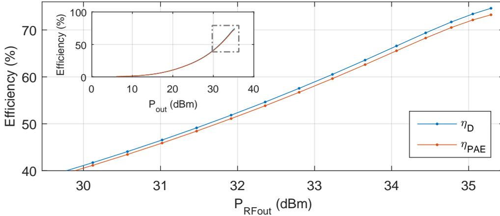
Figure 9.3: Results for efficiency following from the test in Fig. 9.2. The mini-figure shows the corresponding full efficiency characteristic.
