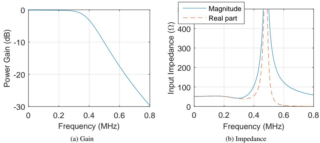
Figure 4.6: 5-pole LC low-pass filter simulations from ADS including parasitic effects. (a) Gain simulation. (b) Input impedance, which is equal to the output impedance.
