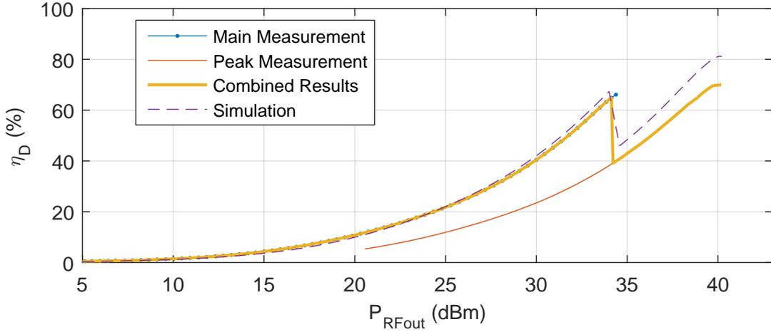
Figure 9.5: Comparison of drain efficiency measurement and simulation for a varying bias interpolating supply PA biased at 28 V peak transistor drain voltage.
