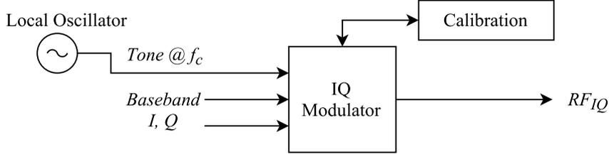
Figure 5.1: Simple overview of the RF signal generation subsystem.
