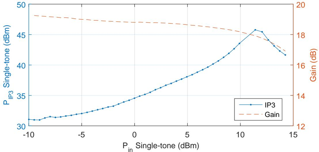
Figure 9.7: IMD measurement for the main transistor of the varying bias interpolating supply PA biased at 28 V peak transistor drain voltage.
