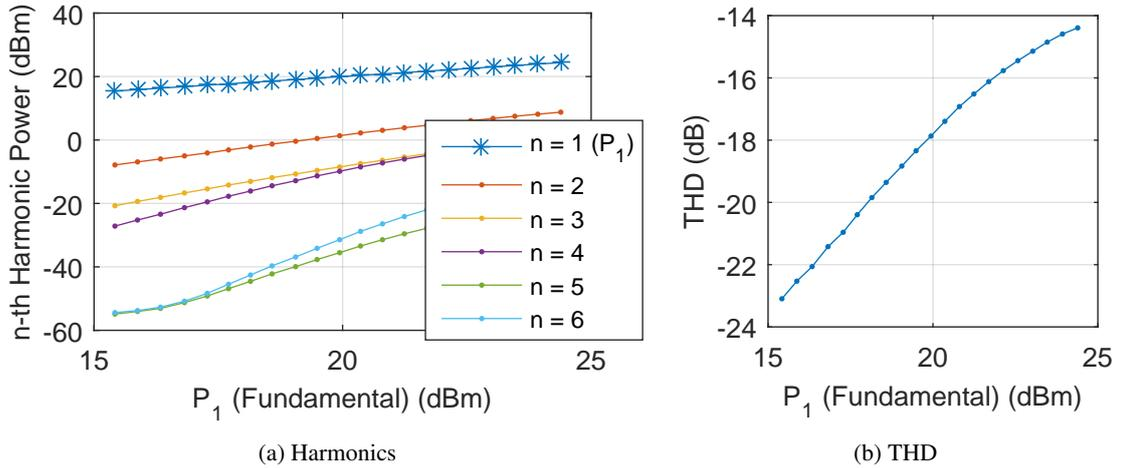
Figure 9.6: THD results,  $P_1$  is the fundamental (100 MHz) output power. (a) Power of harmonics. (b) THD.
