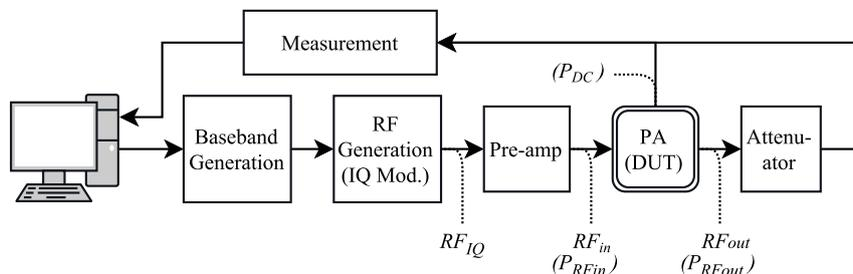
Figure 3.1: Abstracted overview of the entire PA test system and the signal name conventions.
