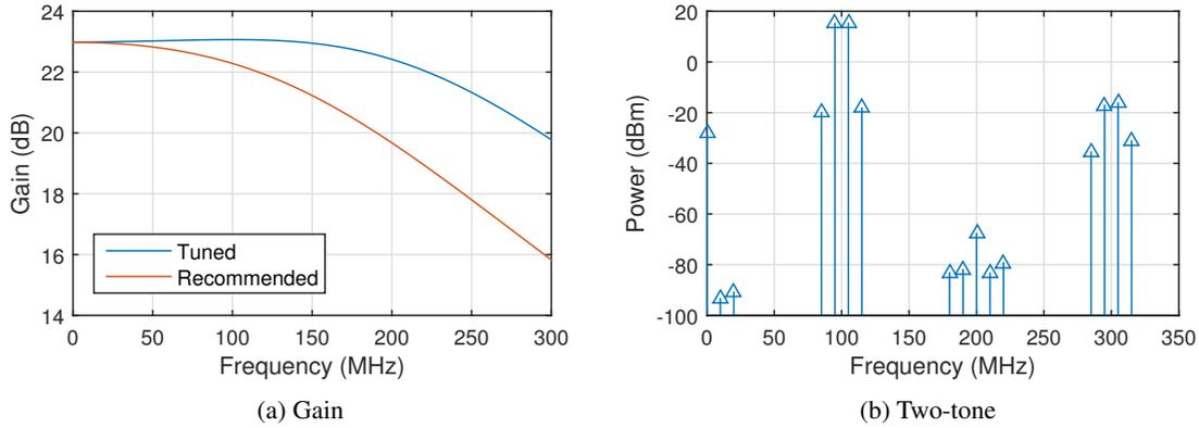
Figure 6.3: Simulation results for a 23 dB CFA. (a) Gain with both the recommended and tuned resistor values. (b) Two-tone signal and its harmonic and intermodulation products.
