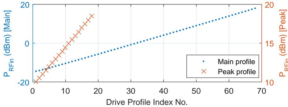
Figure 9.1: Two drive profiles generated for a PA operating in nominal (main) or peak power modes.
