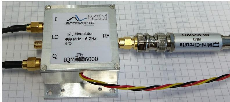
Figure 5.3: IQ modulator and 108 MHz low-pass filter used in this project.
