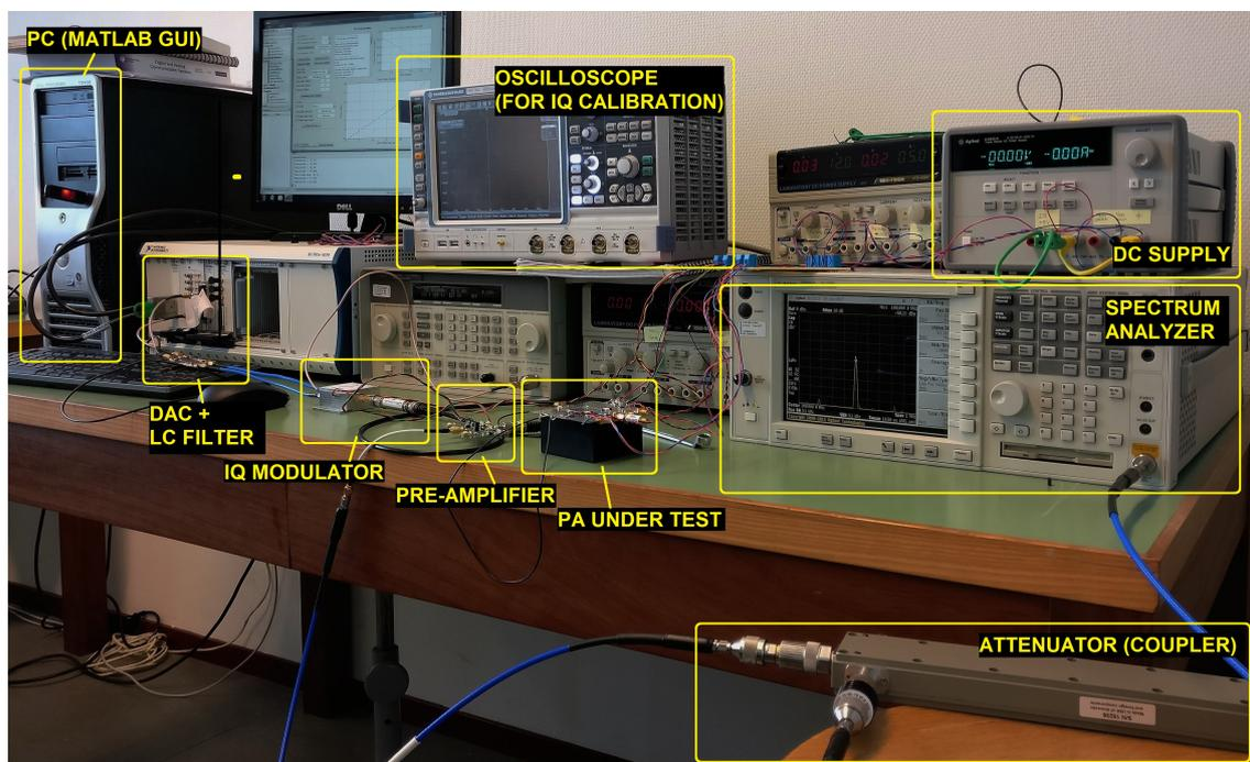
Figure 8.3: Final PA test system hardware with each subsystem designated.
