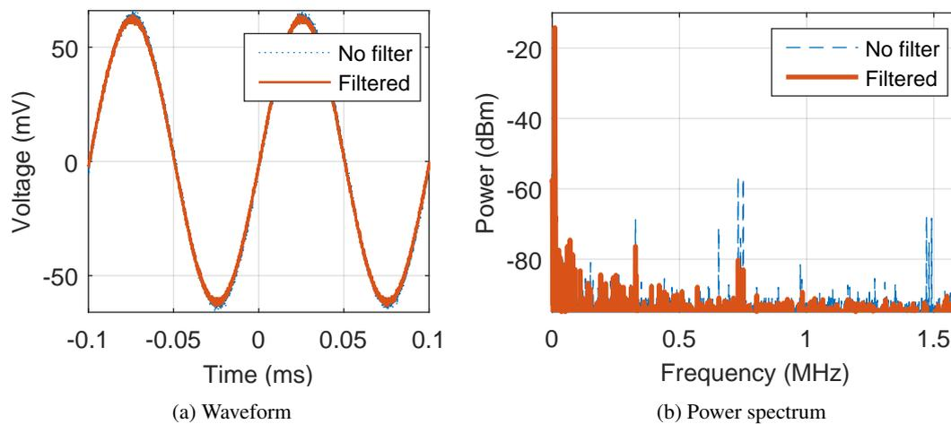
Figure 4.9: 10 kHz sine wave measured at the output of the realized LC filter at a 740 kSa/s output sample rate compared to the no-filter case. (a) Part of the waveform measured. (b) Power spectrum.
