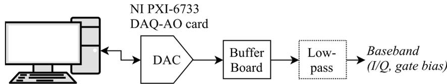
Figure 4.1: Simple overview of the baseband signal generation subsystem.
