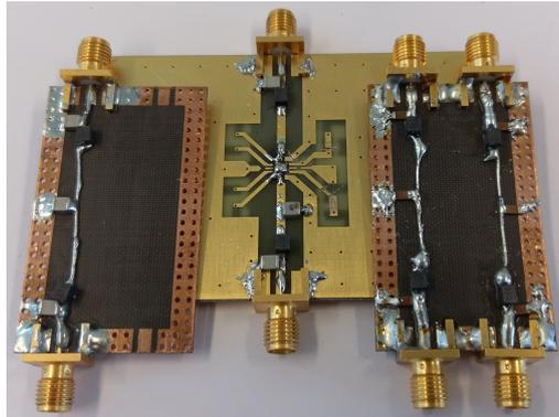
Figure 4.7: Four realized prototype LC filters, each comprising two inductors in the direct path and three capacitors to ground in  $\pi$ -topology.
