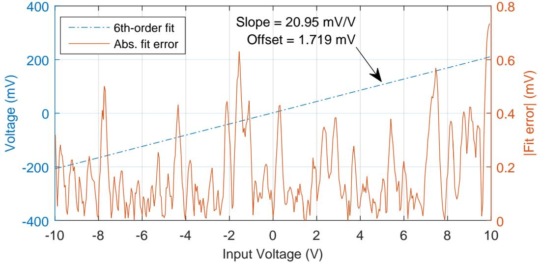
Figure 4.4: Buffer board gain and voltage offset estimated from the fitted mean voltage measurement data with the fit error for justification of the 6th-order polynomial fit.
