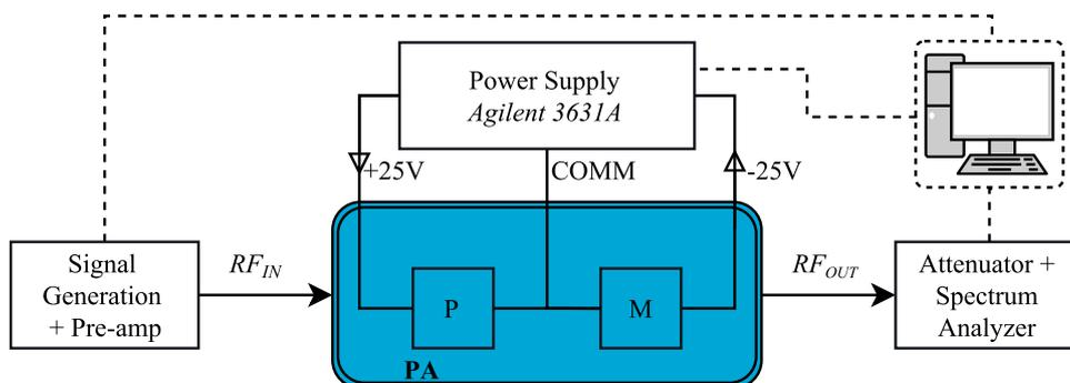
Figure 8.1: Simplified overview of DC power measurement and the PA test system when in measuring and monitoring phase. P and M stand for the peak and main transistors in the interpolating-supply PA family.
