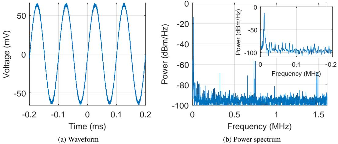
Figure 4.5: 10 kHz sine wave measured at the output of the buffer board at a 740 kSa/s output sample rate. (a) Part of the waveform measured. (b) Power spectrum with a zoomed in view.
