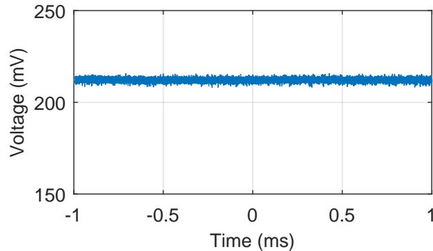
Figure 4.3: Waveform captured by the oscilloscope at the buffer board output with the DAC at maximum positive output voltage. The measured peak-to-peak noise amounted to roughly 10 mV.
