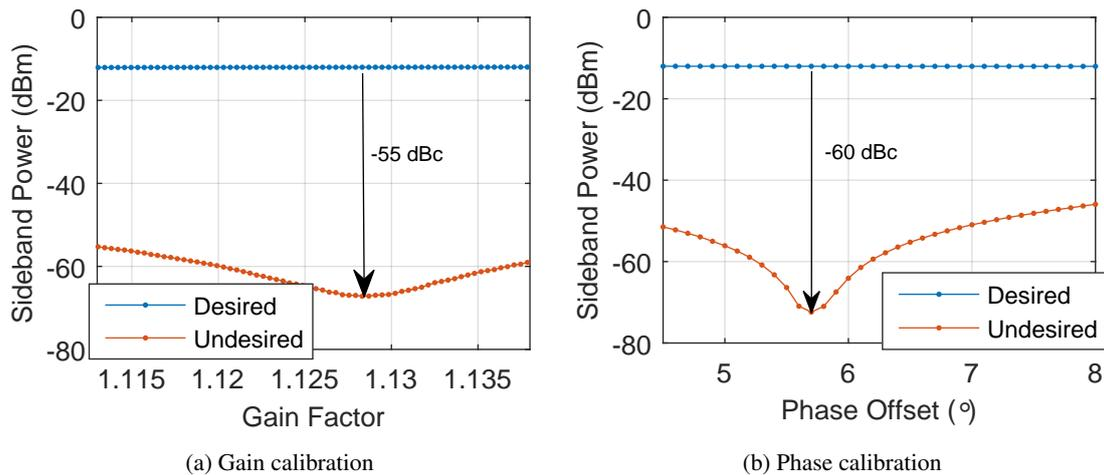
Figure 5.6: Calibration results for USSB with a 10 kHz baseband harmonic. (a) Calibration for gain imbalance. (b) Calibration for phase mismatch.
