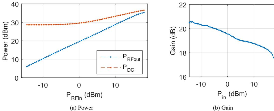
Figure 9.2: PA [2] test results using the main drive profile in Fig. 9.1. (a) Monitored  $RF_{out}$  and DC power. (b) Corresponding computed gain.
