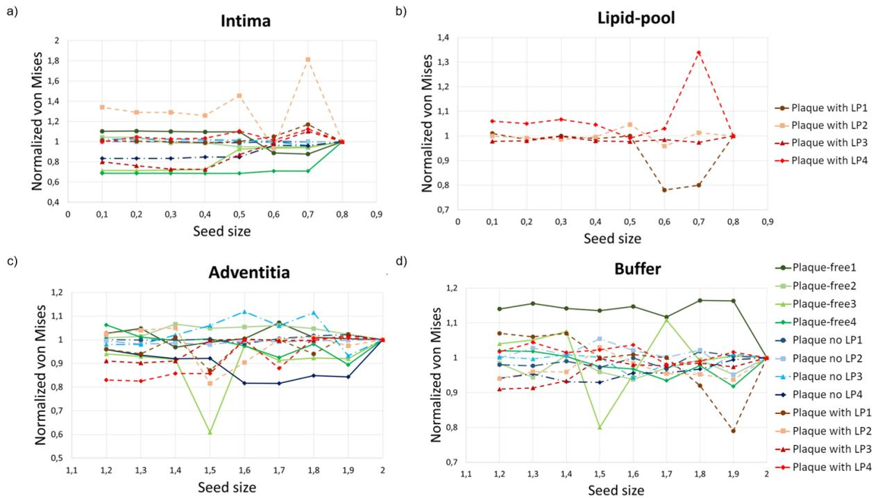
Figure 14: Mesh convergence analysis for: **a)** intima; **b)** lipid-pool; **c)** adventitia; and **d)** buffer.
