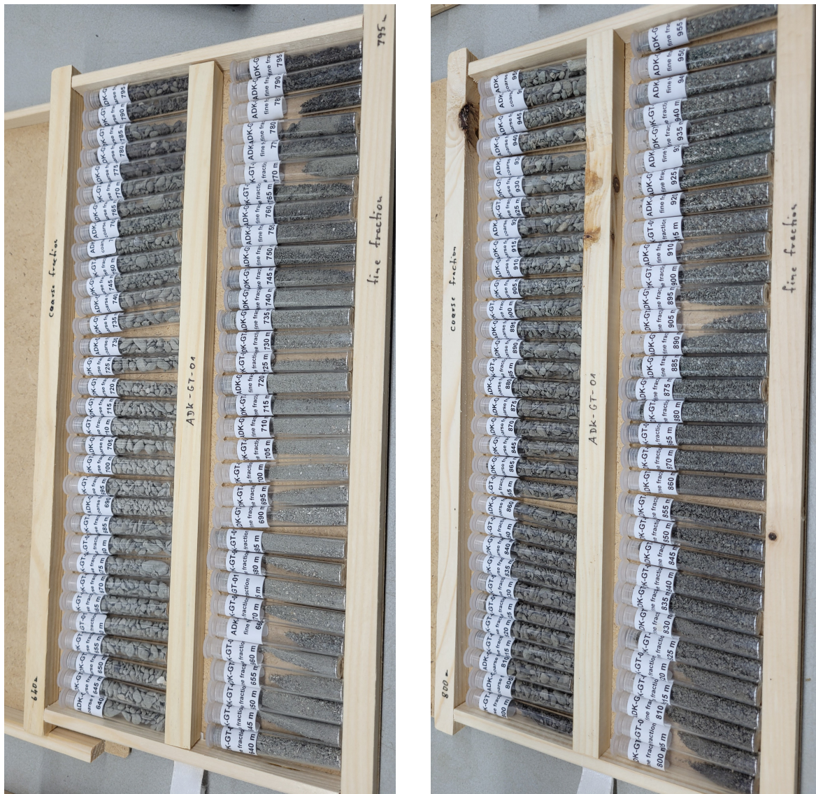
(a) Cutting samples from 640 to 795 m depth (b) Cutting samples from 800 to 955 m depth
