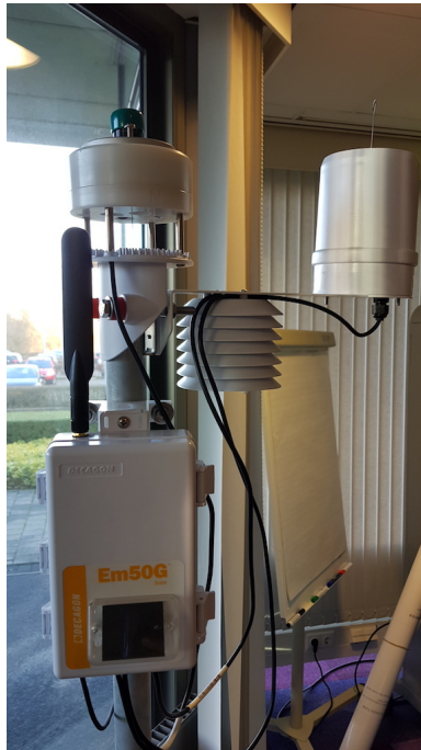
Figure 5.: TAHMO station with a rain gauge sensor module on the top right, used to provide rainfall annotations for the acoustic sensor.
