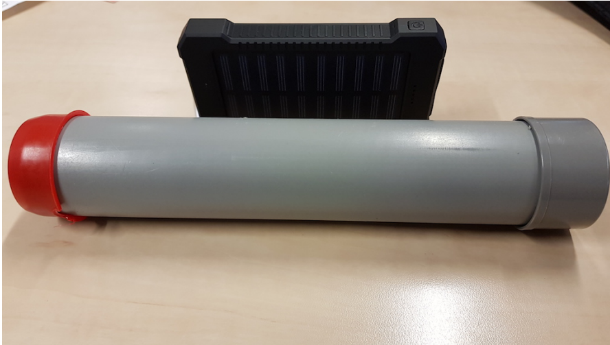
Figure 4.: Acoustic sensor. From left to right: Red speciecap with microphone glued on the inside, PVC pipe where electronics are suspended, PVC bottom cap. In the back is a solar kit(solar panel, battery, USB ports) to provide electronics with power
