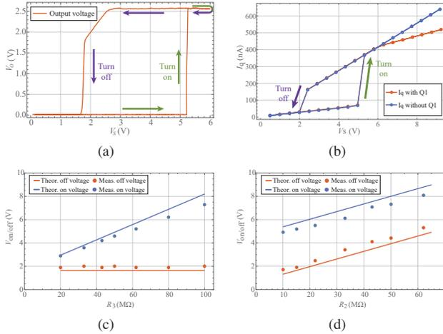
Fig. 5: (a) Output voltage, and (b) quiescent current under storage voltage sweep. Theoretical and measured on/off voltages under different (c)  $R_3$  and (d)  $R_2$ .
