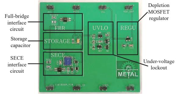
Fig. 4: Evaluation PCB of the proposed power management circuit.
