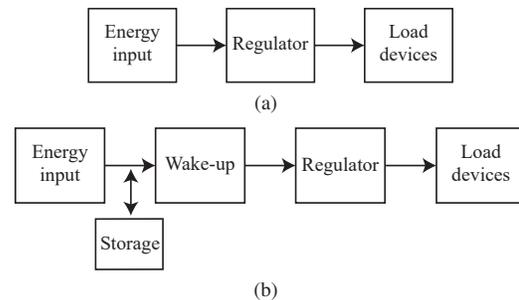
Fig. 1: Power supply architecture of (a) general IoT devices, (b) battery-free IoT devices.
