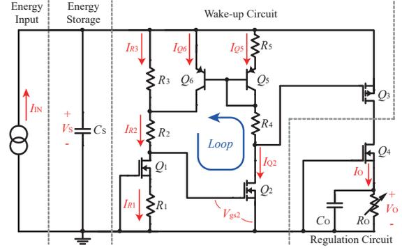
Fig. 2: The proposed power management circuit.
