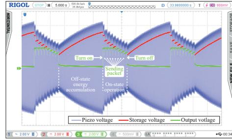
Fig. 6: Waveform in operation when using the piezoelectric source and FBR as the ac/dc interface circuit.
