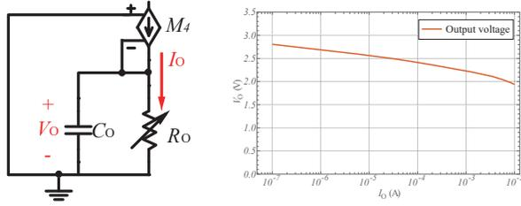
Fig. 3: (a) The proposed power management circuit. (b) The output voltage versus output current with BSS159N.
