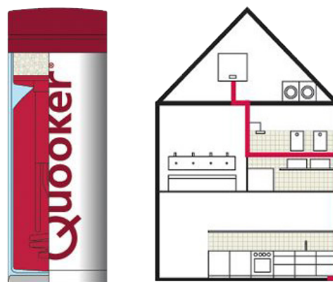
Left: the high-vacuum insulation. right: a conventional way of heating up water
