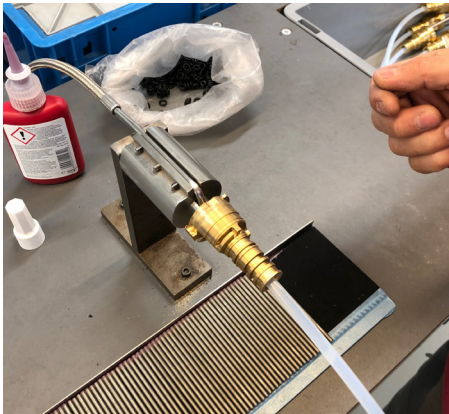
Step 1: attaching the hose and screw shaft into the core component (paddenstoel) of the tap.
