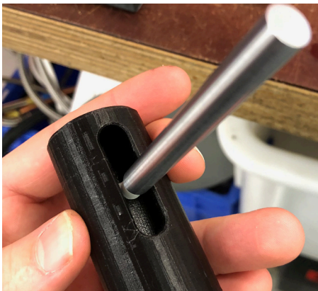
An iteration of prototypes in which different principles of the 'tilt' positioning has been tested. (in this case a horizontal moving handle)
