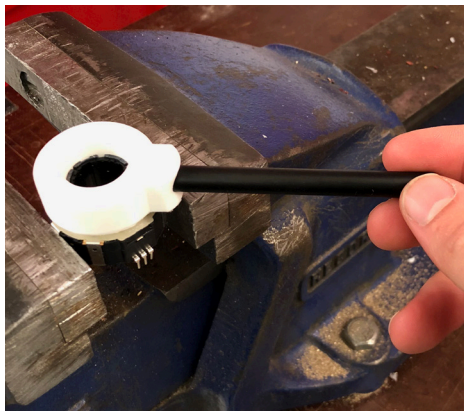
Testing the handle which is attached to a rotary encoder.
