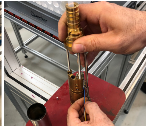
Step 3: combining the two core components of the tap with the screw shaft.
