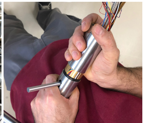
Step 9: attaching the housing (down).
