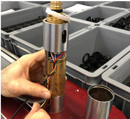
Step 4: attaching the first housing (top) and position the wiring.
