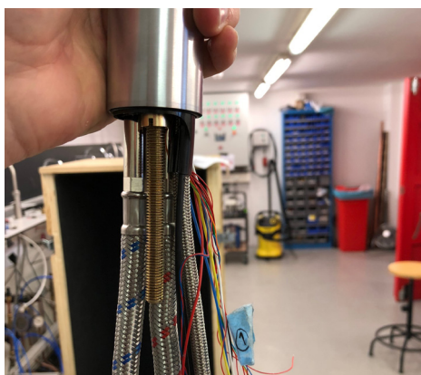
Step 11: attaching the cold and warm hose.
