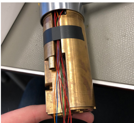
Showing the cavity used to direct all the wiring.
