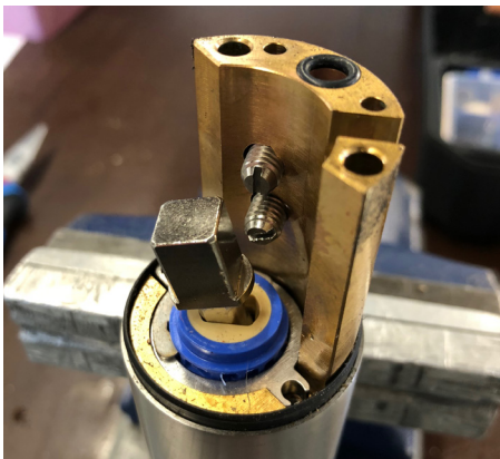
A view on the inside top where the ball spring plunger is attached.
