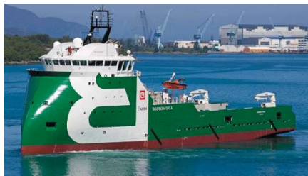
Figure 4-6. The Bourbon Orca: The First X-bow ® , Diesel Electric Anchor Handling vessel
