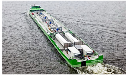
Figure 4-5. The Greenstream: The first 100%, LNG-powered inland shipping vessel
