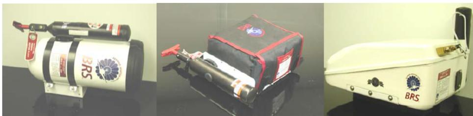
Figure 12.2: Ballistic parachute systems from left to right: the canister, the soft pack and the VLS [57]
