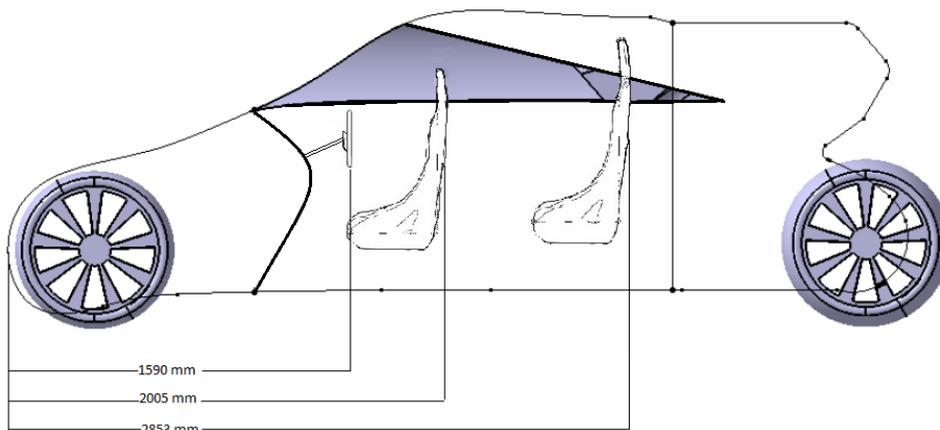
Figure 10.1: Seating configuration inside the vehicle
