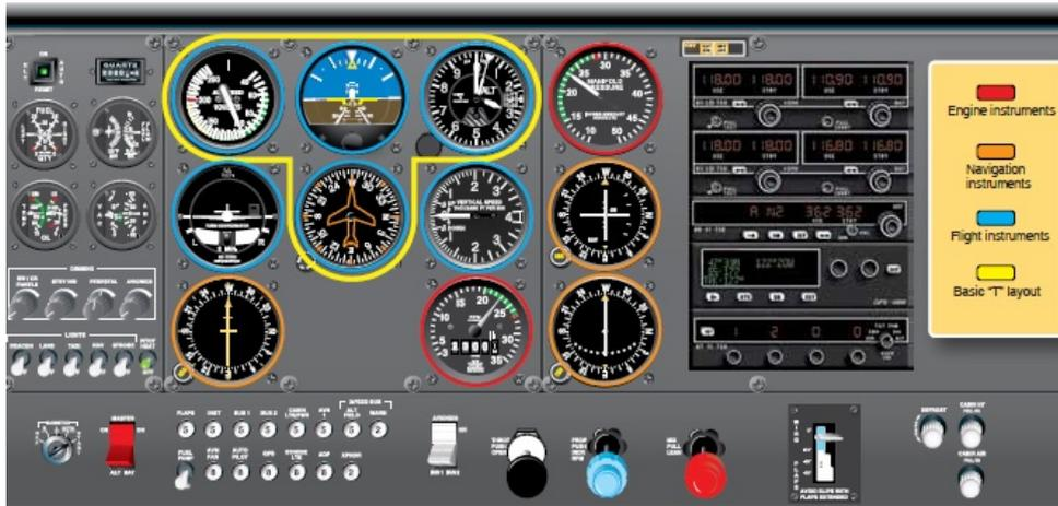
Figure 23.2: Analog cockpit layout [86]
