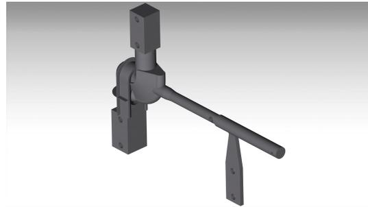
Figure 21.5: Front joint when attached
