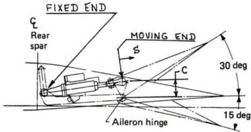
Figure 16.3: Typical actuator-to-surface installation [47]
