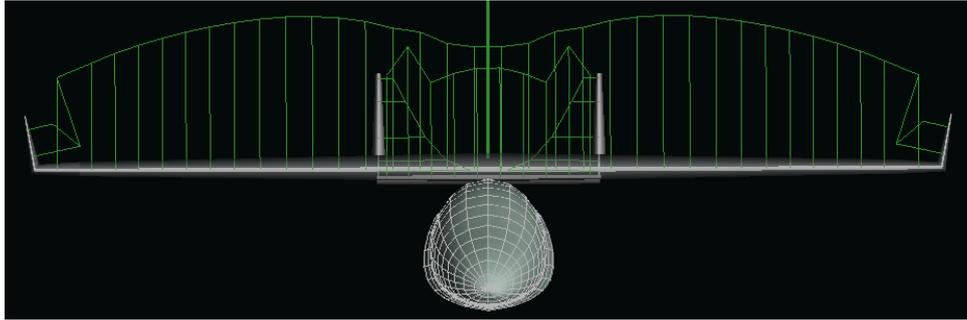
Figure 30.3: Lift distribution of Volucrem in flight
