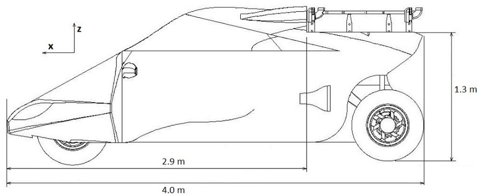
Figure 19.2: Side view of the attachment system with respect to the car dimensions
