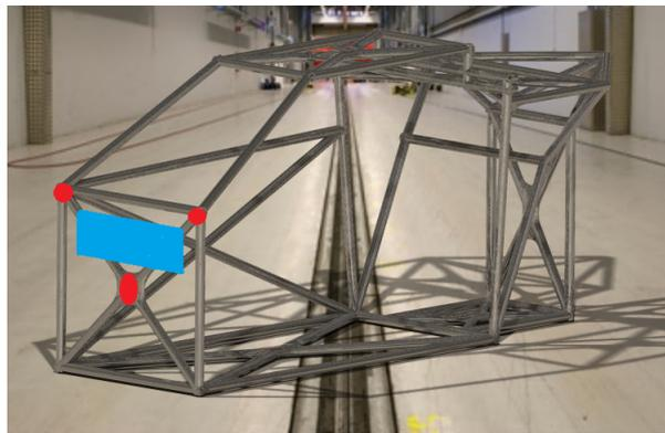
Figure 12.3: The position of the BRS-172 and the harness connection on the safety cage
