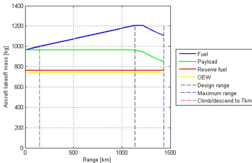
Figure 18.2: Payload range diagram at maximum speed
