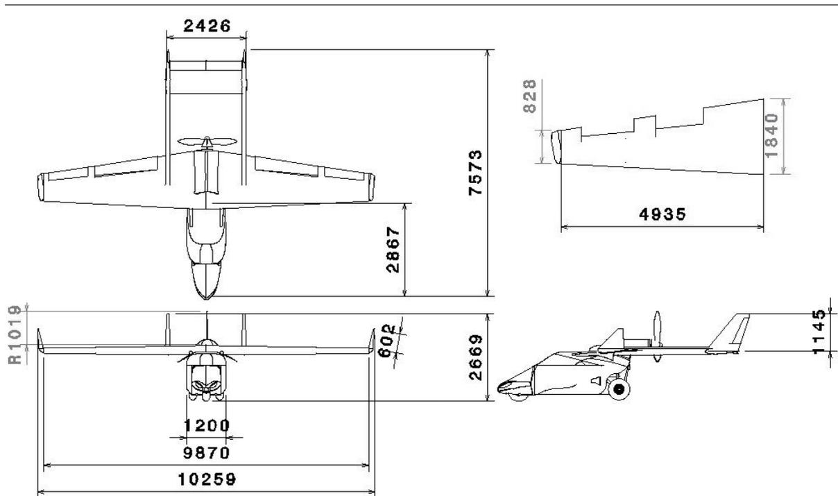
Figure 13.2: Complete flight module with dimensions in mm
