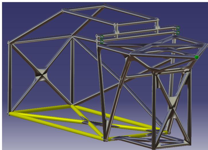
Figure 8.2: Load and clamping placements for the FEM of the roll cage in the extreme manoeuvring case
