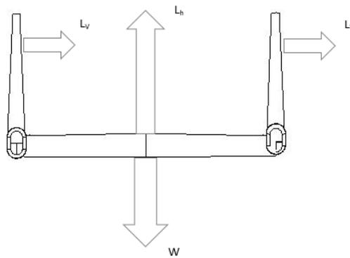
Figure 14.2: Forces on the tail applied
