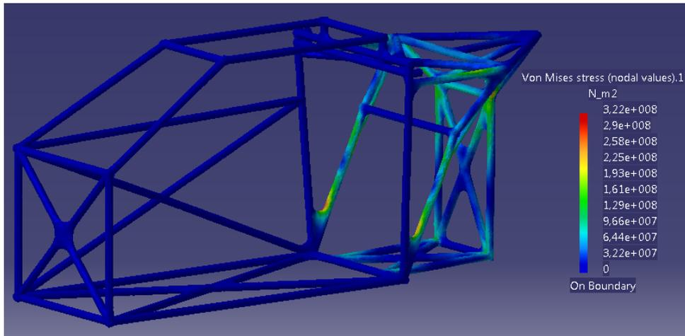
Figure 8.6: Front side view of FEM results of the roll cage for the extreme landing case
