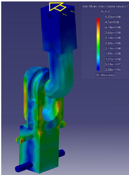
Figure 20.3: FEM  $x=25\text{ kN}$  (wing forward)
