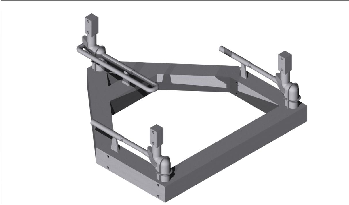
Figure 21.8: Attachment system including parts of the safety cage
