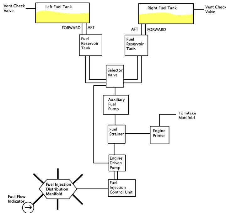
Figure 15.4: Pump driven fuel system for the flight module
