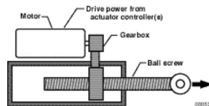
Figure 16.2: Electromechanical Actuator[72]
