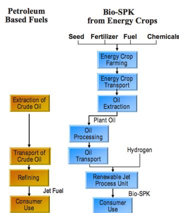
Figure 15.3: Fuel processing flow diagram [67]
