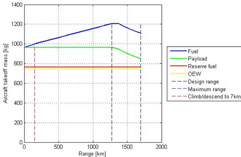
Figure 18.1: Payload range diagram at cruise speed
