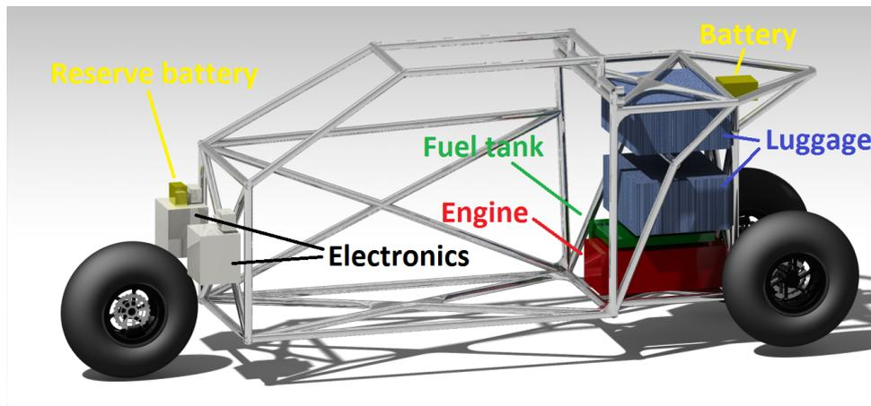
Figure 10.6: Location of the batteries, hand luggage, fuel tank, engine and electronics
