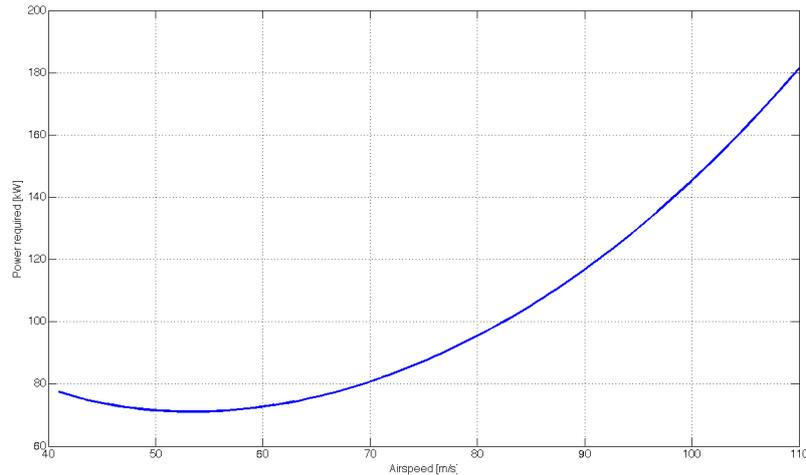
Figure 15.2: Power required versus cruise airspeed
