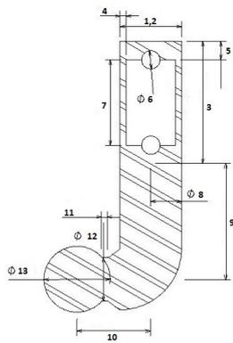
Figure 20.7: Dimension numbering of the ball hook, side view
