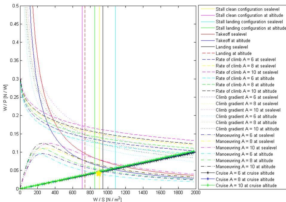
Figure 5.1: Power and wing loading diagram
