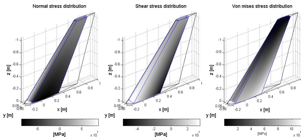
Figure 14.5: Stress analysis of the vertical tail
