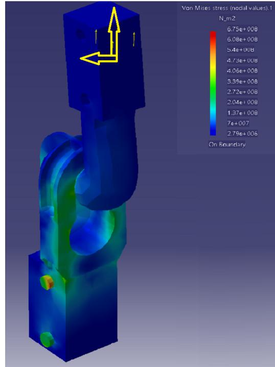
Figure 20.6: FEM  $x=5, y=5, z=30$  kN (tension)
