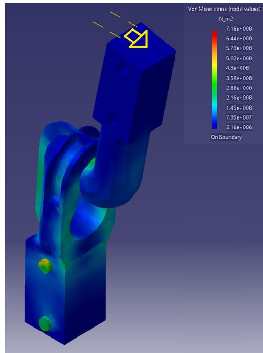
Figure 20.4: FEM  $x=-12\text{ kN}$  (wing backward)
