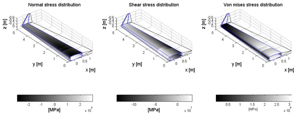
Figure 14.1: Stress analysis for the wing
