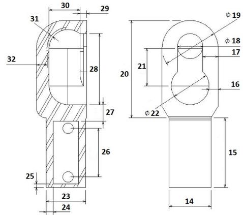
Figure 20.8: Dimension numbering of the socket, left side view, right front view
