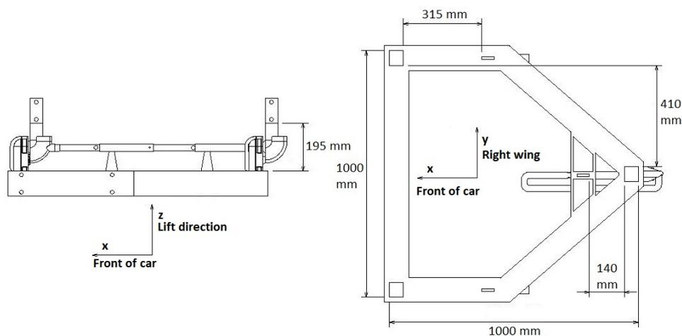
Figure 19.1: Left: Side view of the attachment system. Right: Bottom view of the attachment system
