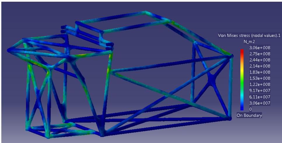
Figure 8.4: Back side view of FEM results of the roll cage for the extreme manoeuvring case
