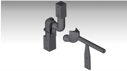
Figure 21.4: Front joint when open
