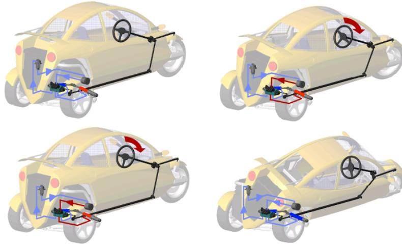
Figure 10.2: Principle of the DVC system [13]
