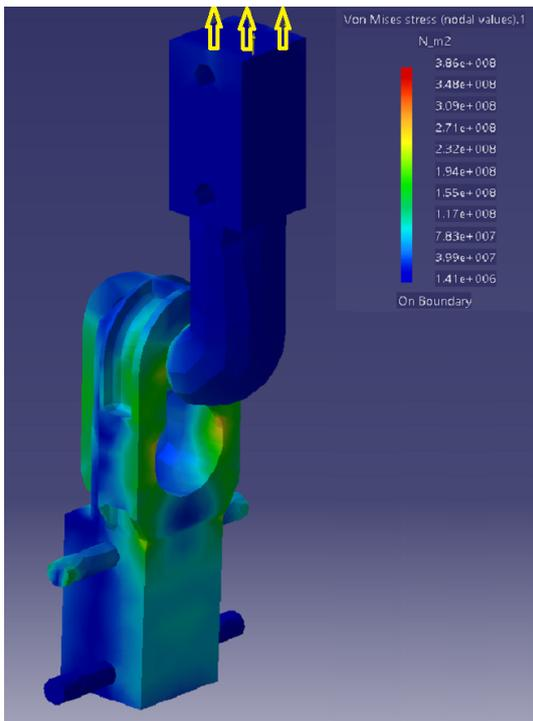
Figure 20.1: FEM  $z=40\text{ kN}$  (tension)
