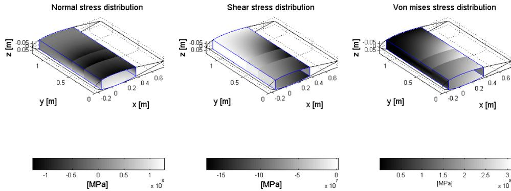
Figure 14.4: Stress analysis of the horizontal tail
