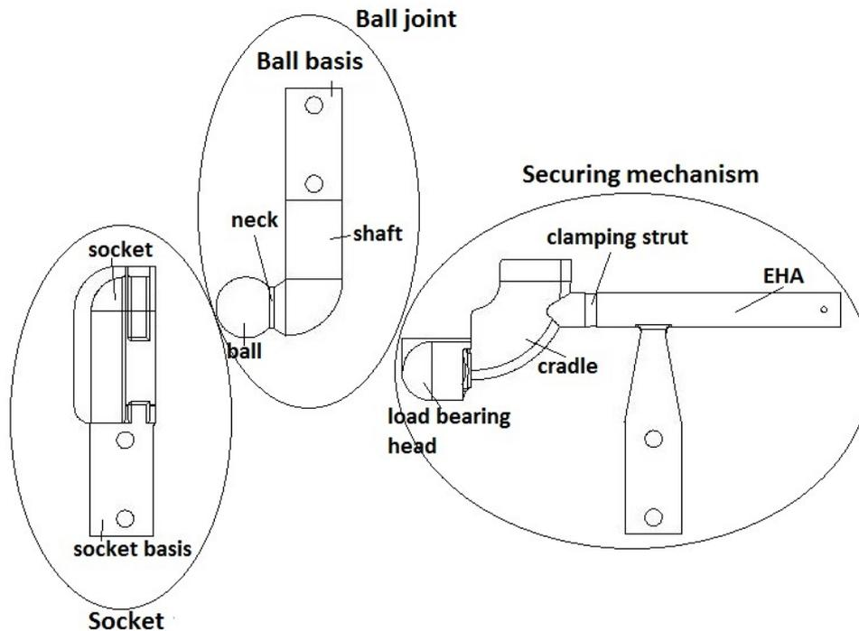
Figure 19.3: Specific names of the attachment joints
