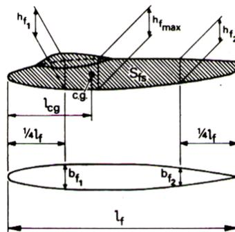
Figure 17.6: Parameters used for determination yaw moment contributions [76]
