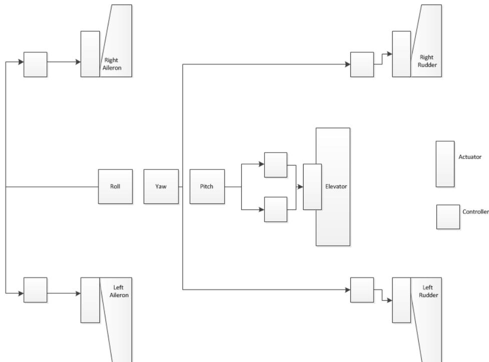
Figure 16.4: Flight Control Schematic
