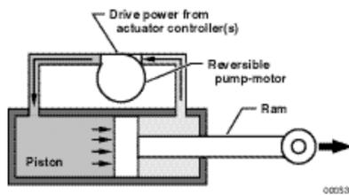
Figure 16.1: Electrohydrostatic Actuator[72]
