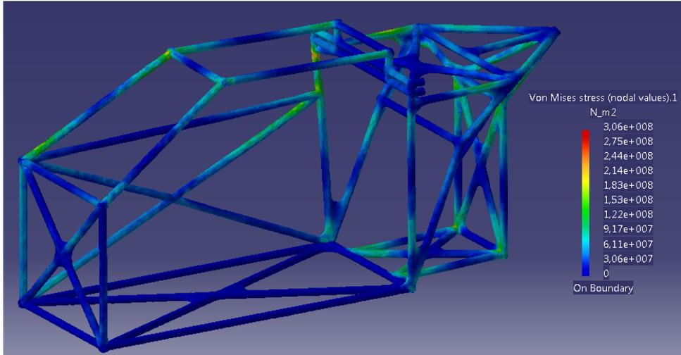
Figure 8.3: Front side view of FEM results of the roll cage for the extreme manoeuvring case
