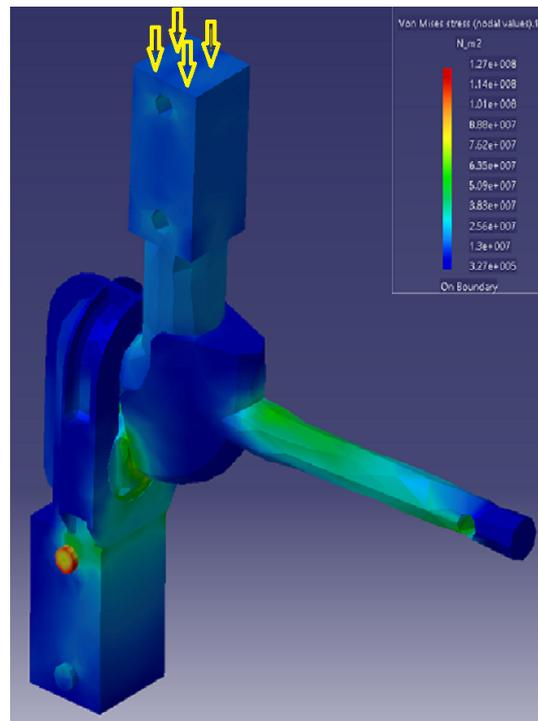
Figure 20.2: FEM  $z=-40\text{ kN}$  (compression)
