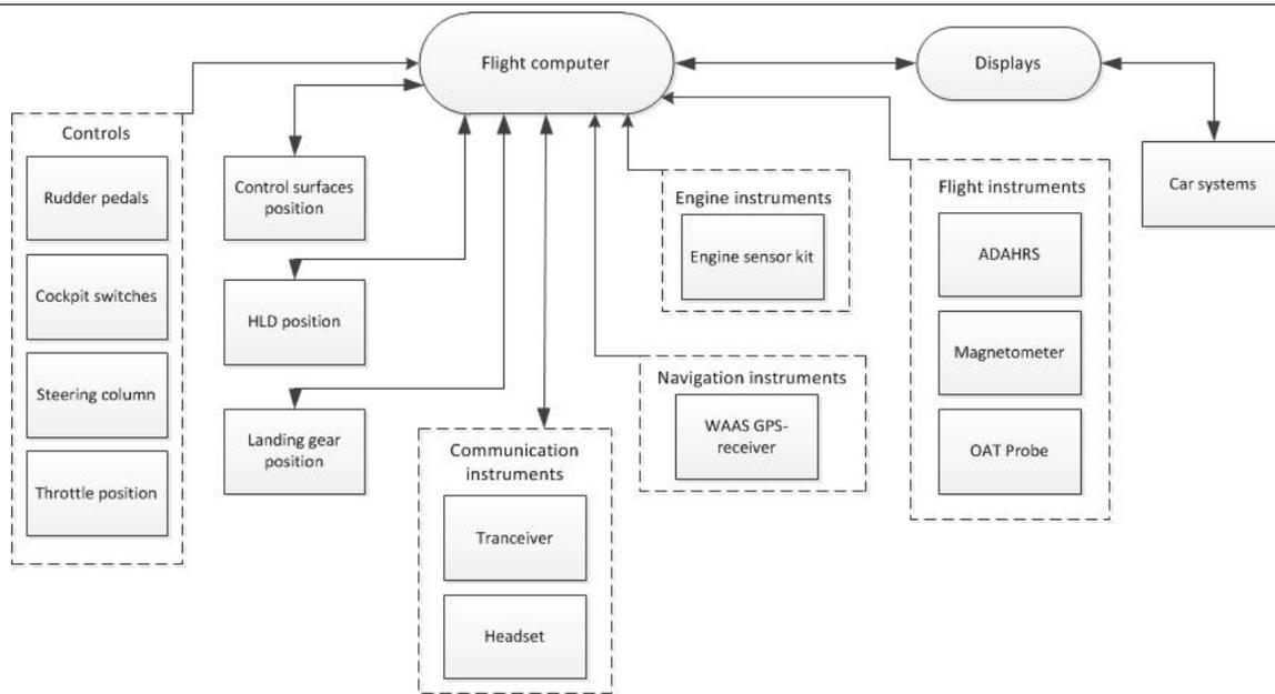
Figure E2: Electronic block diagram of the aircraft electronic systems
