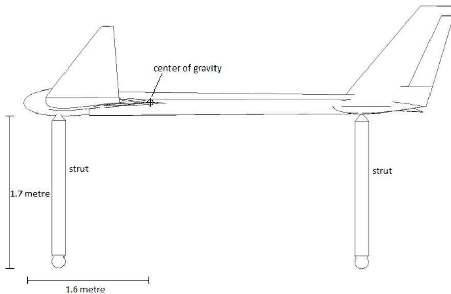
Figure 21.3: Side view of the flight module positioning stage
