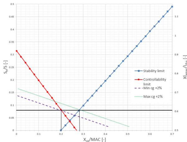
Figure 17.5: Projection of scissor plot and c.g. range
