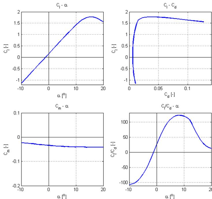
Figure 13.1: Airfoil characteristics at  $Re = 5.13 \cdot 10^6$
