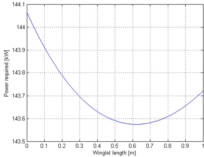
Figure 13.3: Power required versus winglet length
