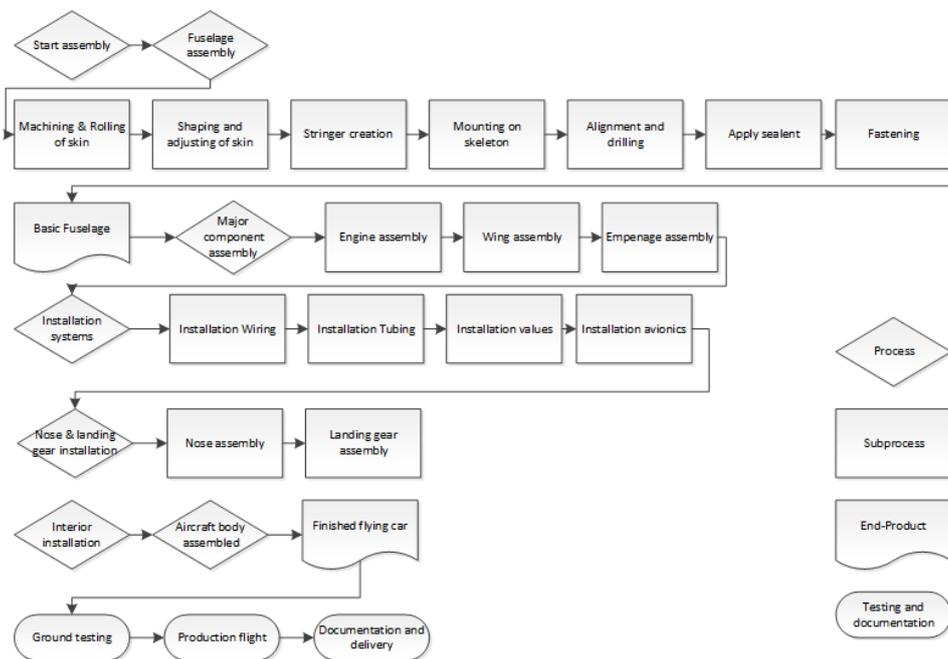
Figure 22.1: Manufacturing, assembly and integration plan
