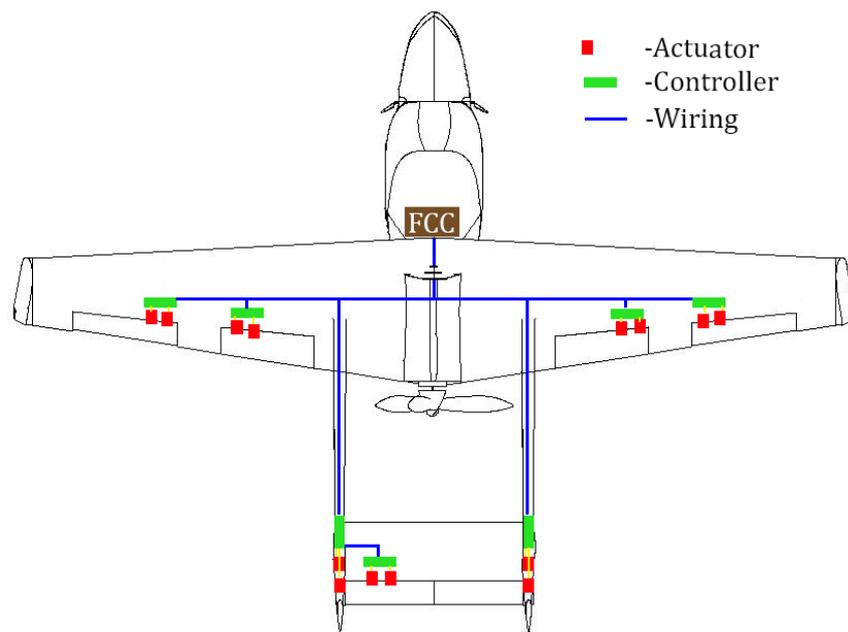
Figure 16.5: Flight control system layout
