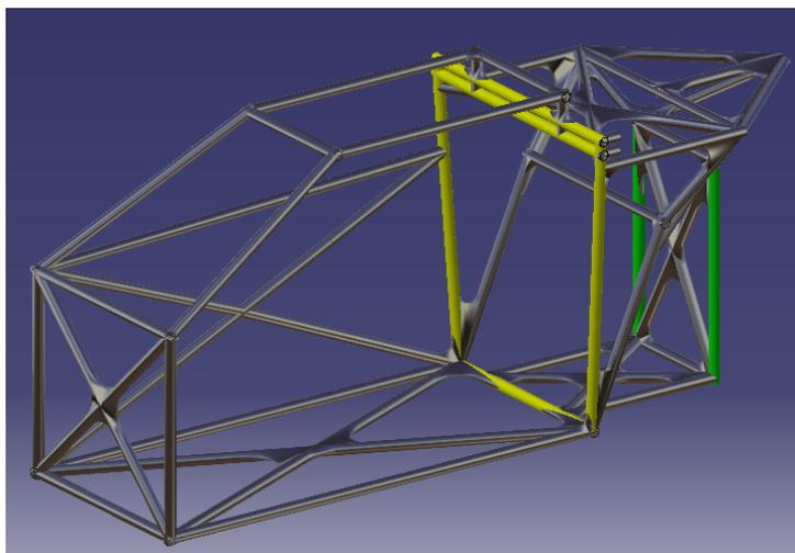
Figure 8.5: Load and clamping placements for the FEM of the roll cage in the extreme landing case
