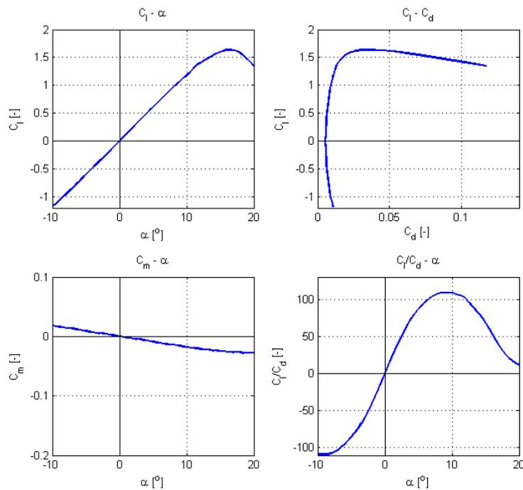
Figure 13.4: Airfoil characteristics at  $Re = 5.13 \cdot 10^6$
