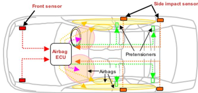
Figure 12.1: Airbag system in a normal car [53]
