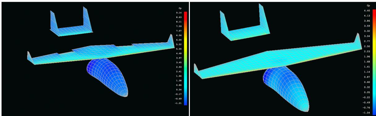
Figure 30.1: Pressure coefficient distribution for an airspeed of  $40 \frac{m}{s}$  and a 7.5 degree angle of attack
