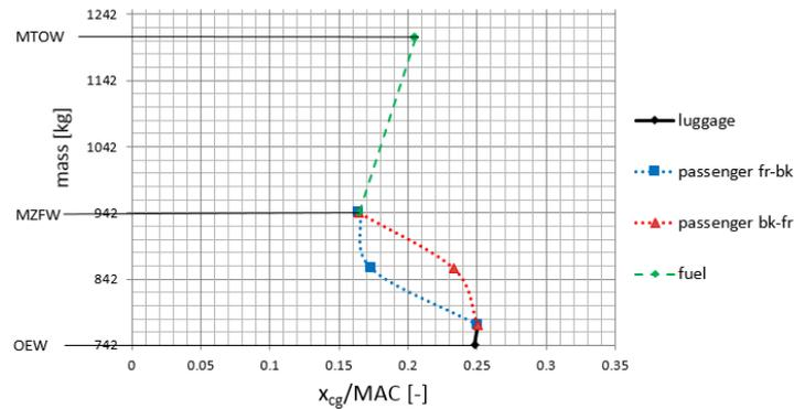
Figure 17.3: Loading Diagram
