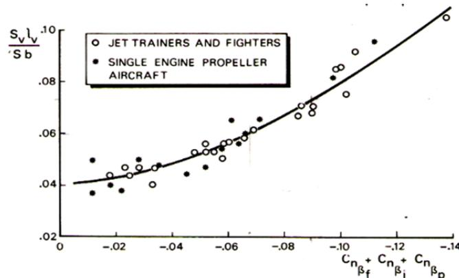
Figure 17.7: Vertical tail sizing jet trainers, fighters and single engine propeller aircraft [76]
