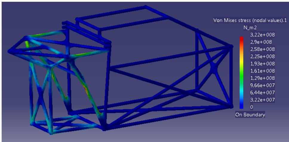
Figure 8.7: Back side view of FEM results of the roll cage for the extreme manoeuvring case
