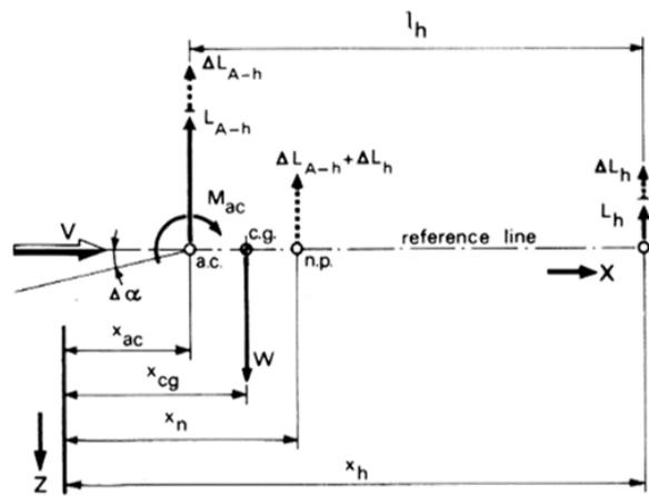
Figure 17.1: Forces and moments for longitudinal stability [75]
