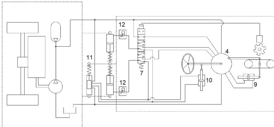
Figure 10.4: Advanced DVC system in a carver [14]
