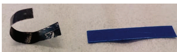
Figure 4.11: Bending of an actuator when removed from PP layer
