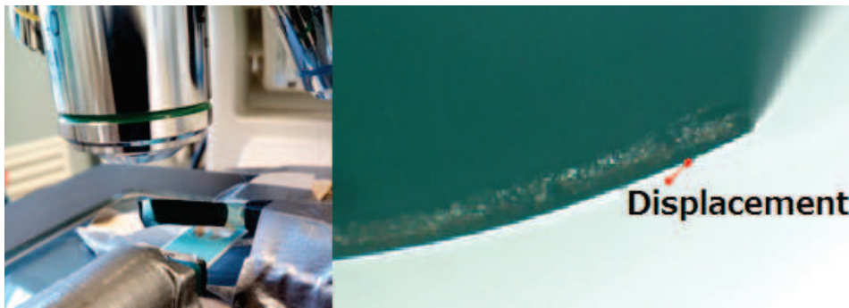
Figure 2.4: Experimental setup of a TOPAS-gold-PPY/NaDBS actuator beam,designed to measure the displacement at micro scale.
