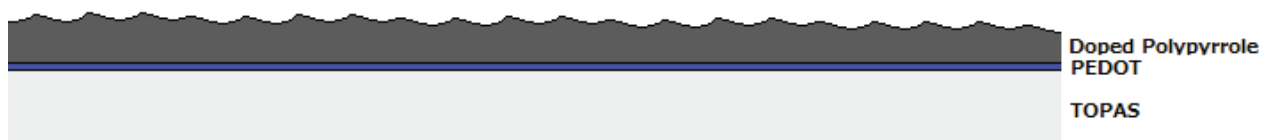
Figure 2.1: Active layers of the all conducting polymer microvalve actuator systems.
