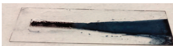
Figure 4.9: patterning using spin coating PEDOT while mask of PP
