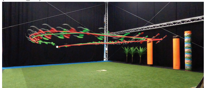
Fig. 1: A comparison of a circular flight path between the proposed controller (green) and a classical PID controller (red)
