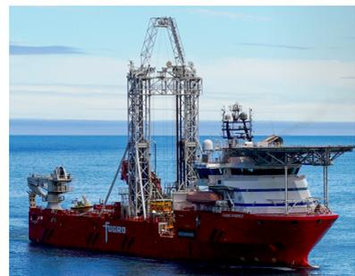
(b) Geotechnical Survey Vessel - SYNERGY
