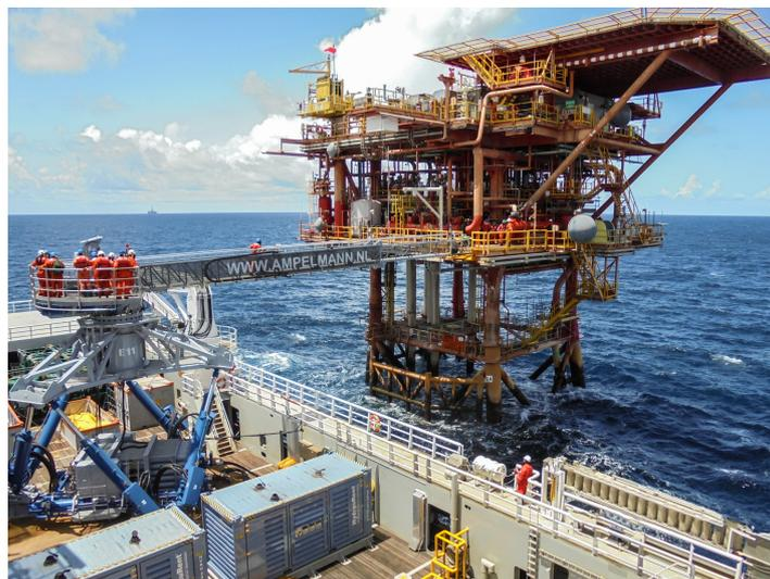
**Figure 1-1:** Ampelmann E-type during offshore operation
