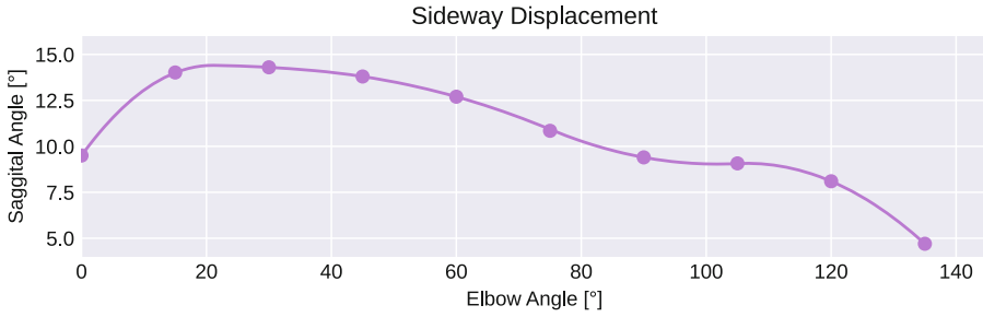
Fig. 8. Sideway displacement of BICEP for different angles ranging from 0^\circ to 135^\circ with 500 g load condition. For this experiment the BICEP was mounted sideways to the table. The plot shows a maximum displacement of 14.3^\circ .
