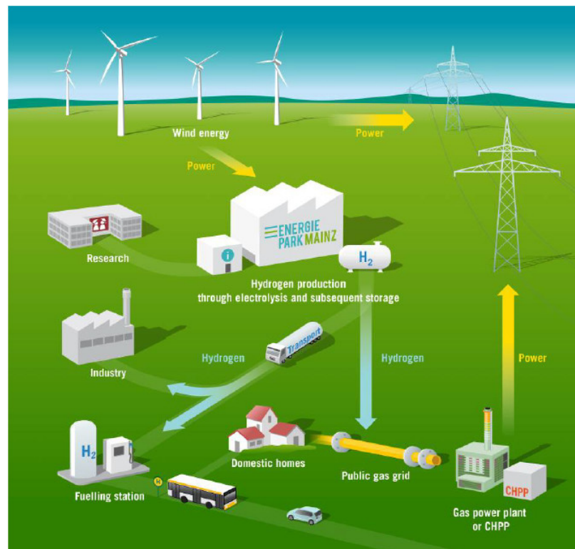
Figure 1.2: An overview of a hydrogen infrastructure with the process of using the excess energy from renewable energy source to generate hydrogen. This generated hydrogen can be used in a gas turbine power plant to generate energy when the energy from the renewable energy sources are not complying with the energy demand. Figure adopted from Zorn [73].
