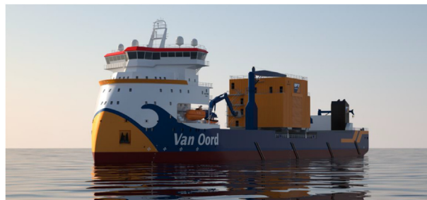
Figure 3 An outcome of the design inquiry: an advanced subsea rock installation vessel. New insights on enhancing innovativeness of complex objects were put to practice during the initial design stages
