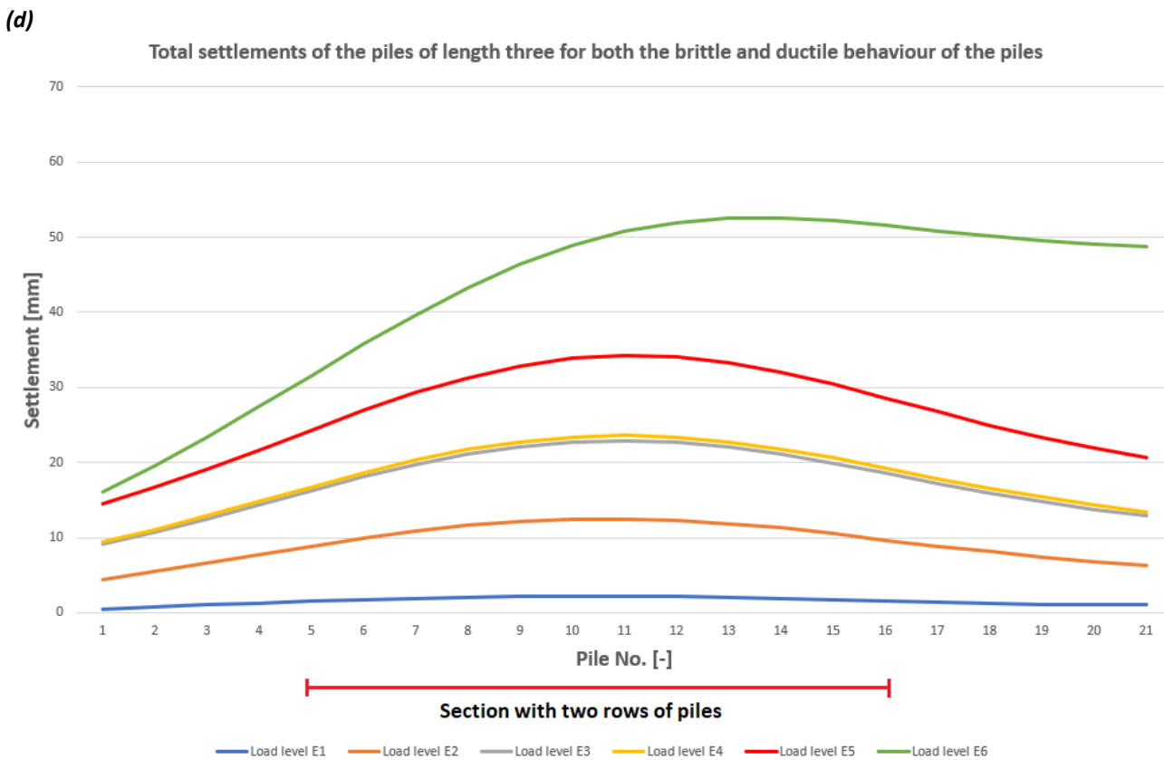
Figure 6.22: total settlement of the piles for (a) length zero, (b) length one, (c) length two and (d) length three for both the brittle and ductile behaviour of the piles.
