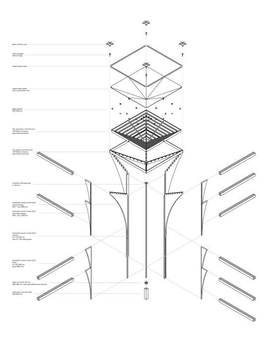
Exploded axonometry of the column and chalice element
