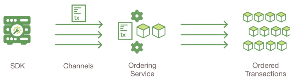
Figure 33: The app sends endorsed transaction proposal to ordering service to create blocks(Transaction Flow, 2021)
