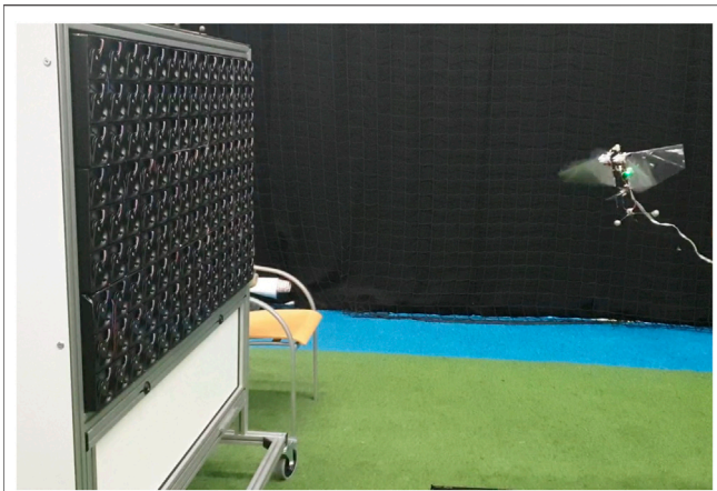
FIGURE 7 | The test setup of free flight experiments of the asymmetric flapping-wing MAV with the low-speed multi-fan wind system.
