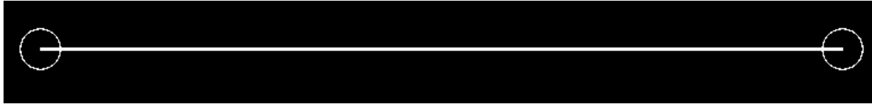
Figure 3-9: Laser cut file of the channel together with the holes. The centers of the holes coincide with the channel ends. The channel length is equal to 40 mm, and the width is equal to 200 \mu\text{m}
