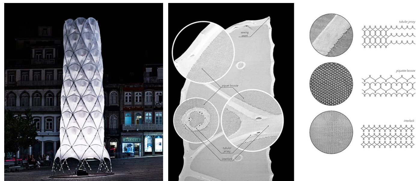
Figure 11. (A) Hybrid Tower (Source: Anders Ingvarsten/ArchDaily), (B) Knit patterns used in the Hybrid Tower textile (Source: CITA/ArchDaily)
