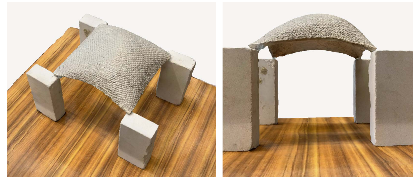
Figure 63. 3D scans of one sample showing the high degree of detail achieved through photogrammetry scanning.
