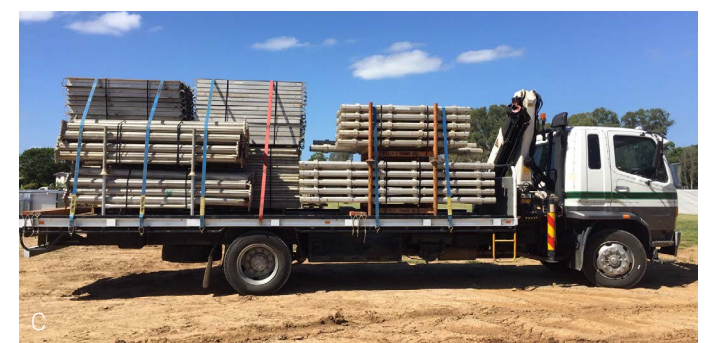
Figure 9. Transportation of textile formwork vs. transportation of rigid formwork. (A) Textile formwork used in KnitCandela being vacuum-compressed for transport in checked luggage (Source: Block Research Group), (B) Luggage used to transport 13 building-scale column formworks (Source: Mark West / C.A.S.T), (C) Typical transport of rigid formwork (Source: Southern Cross Crane)
