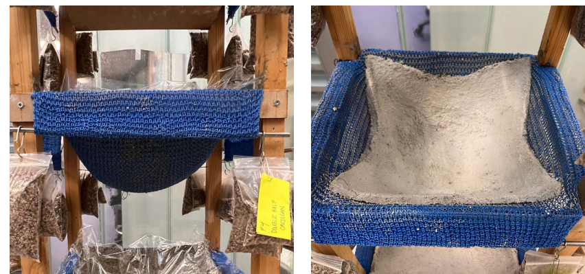
Figure 60. Highly deformed samples on the casting frame.
