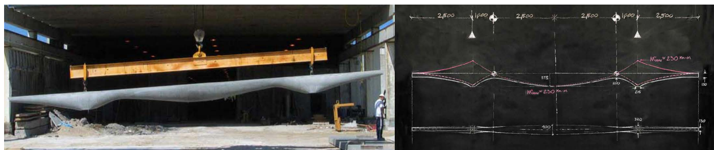
Figure 21. Prototype for a beam whose shape follows the curve of its bending moment by Mark West / C.A.S.T. (Source: Mark West / C.A.S.T.)
