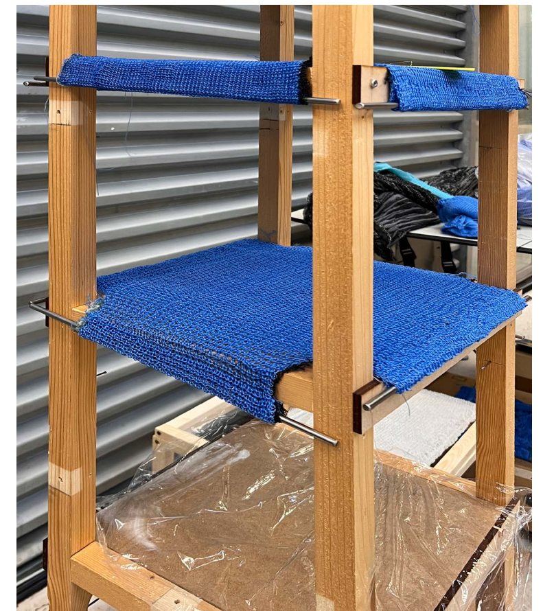
Figure 48. Double Half Cardigan cruciform sample being fitted to the casting frame during the gauge calibration process. Some samples were knit multiple times to achieve precise dimensioning.
