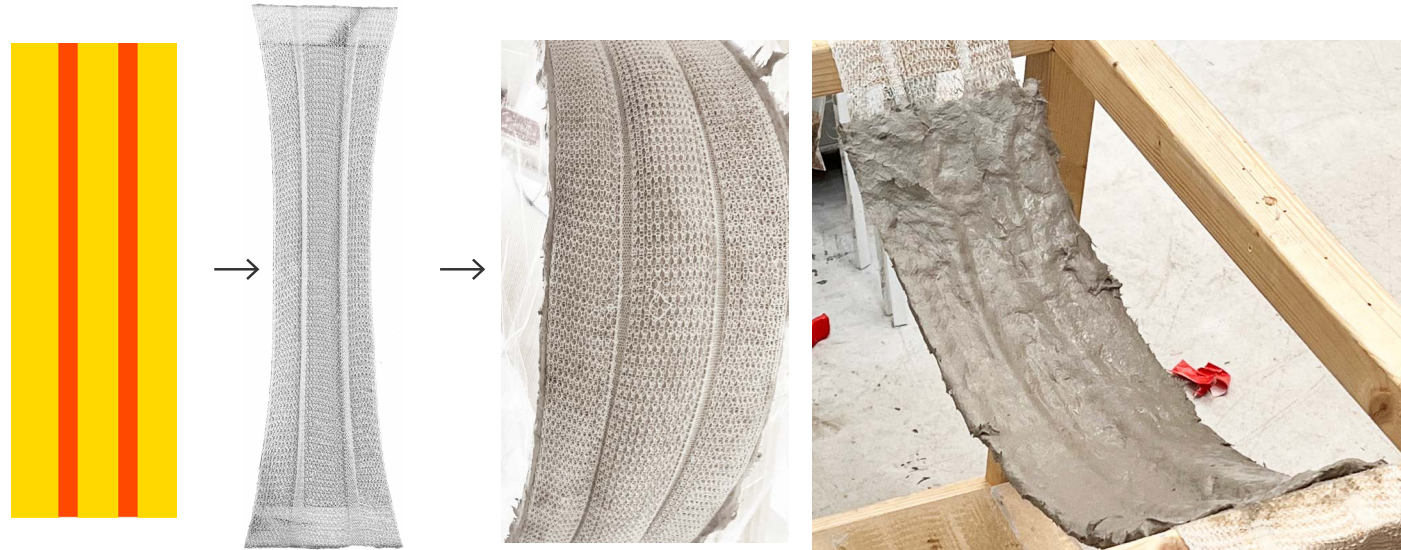
Figure 118. (Left) Desired pattern template shape, (Middle) Actual knit textile, (Right) Alt Stripe textile immediately after casting showing significant deformation and ribbing.
