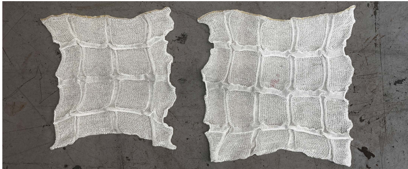
Figure 134. Two versions of the Grid pattern were knitted during the calibration process. The 4x4 grid shown on the left was too small in the weft direction for the casting frame, so another column was added to create the 5x4 grid shown on the right. Although no additional stitches were added in the warp, the addition of this column created an increase in both the weft and warp directions.
