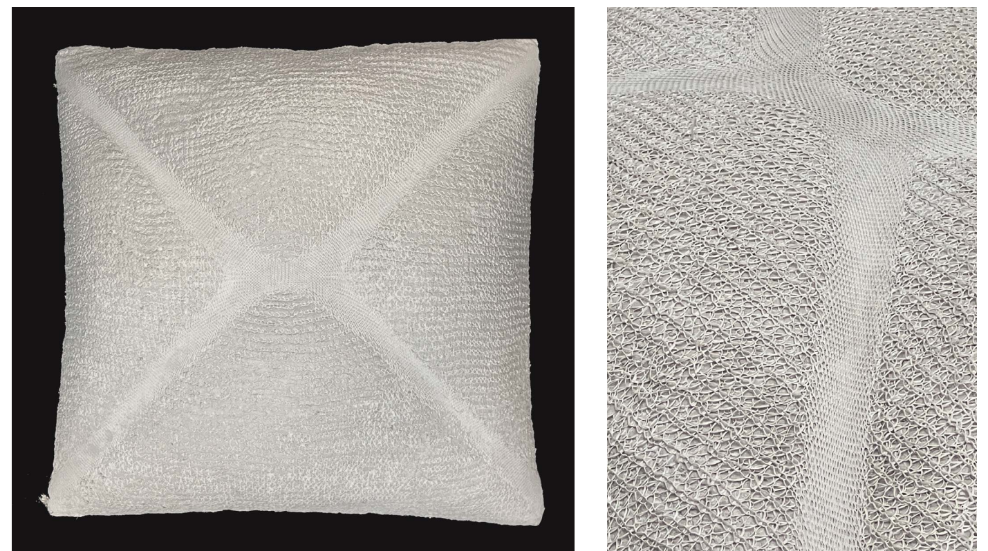
Figure 107. (Left) Plan view of X-shape cast sample, (Right) Close-up view of pattern texture.
