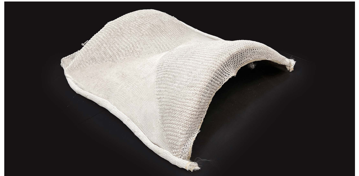
Figure 101. Side view of 4-Quadrant (Alt Supports) casting result prior to textile removal.
