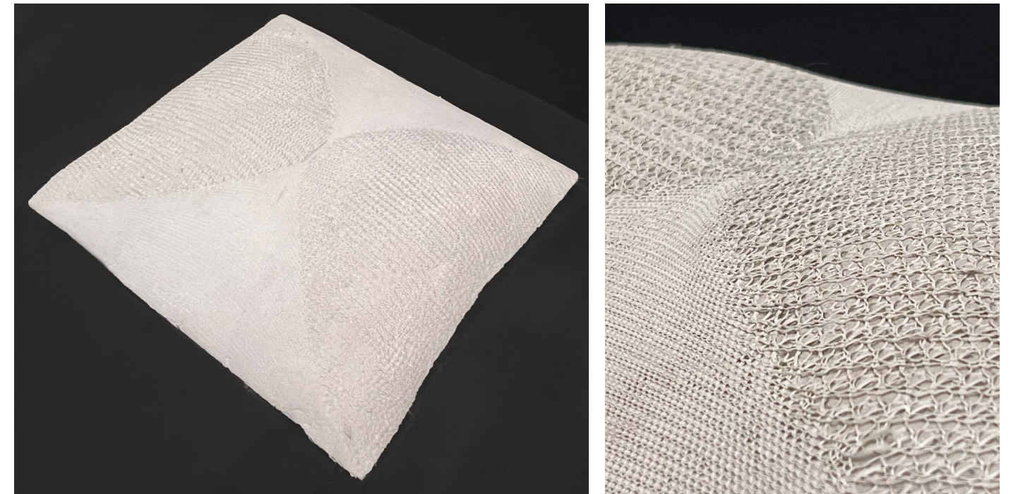
Figure 95. (Left) Perspective view of 4-Quadrant casting result after removal of textile, (Right) Close-up view of surface texture prior to removal of textile.
