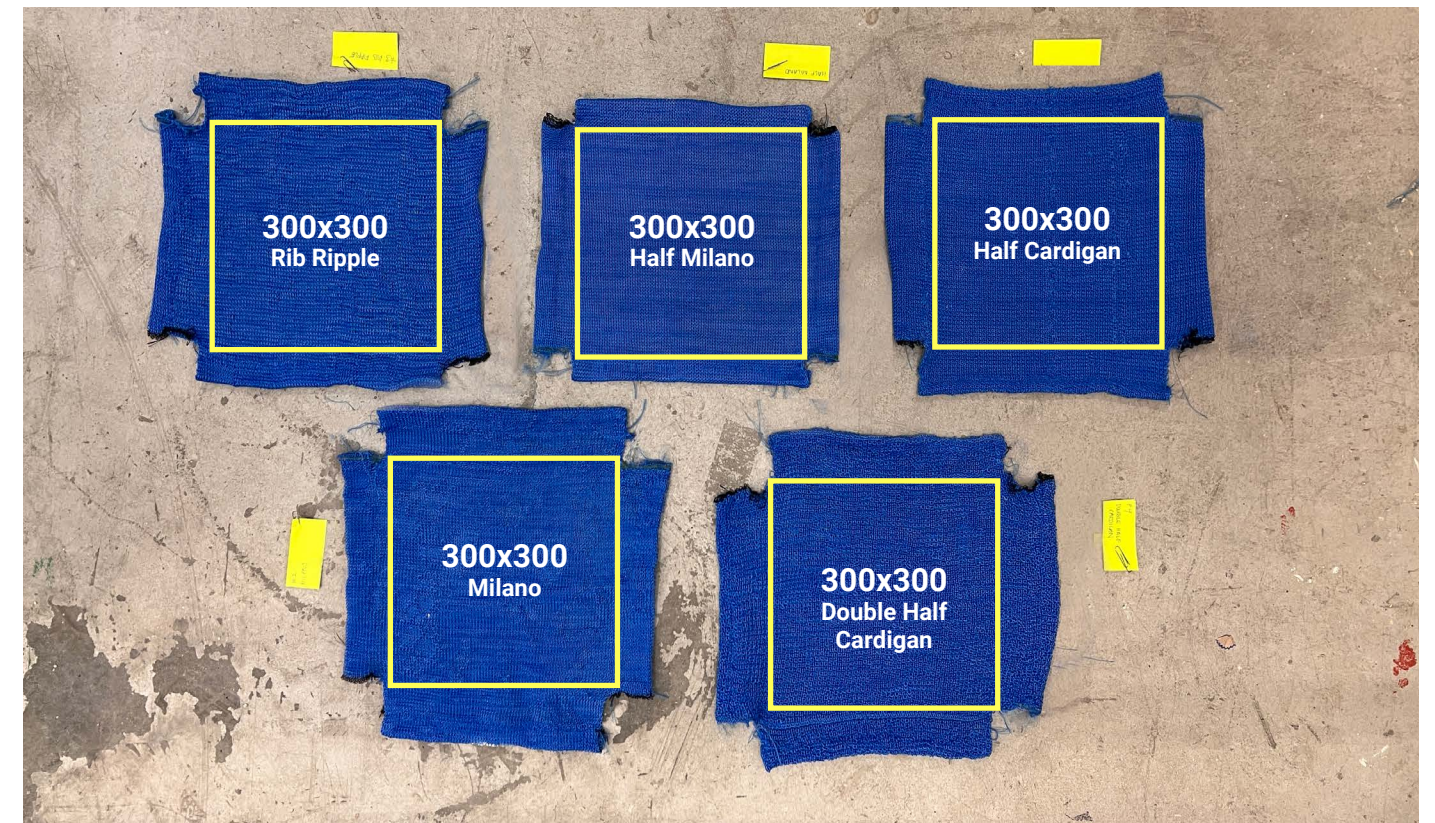
Figure 46. Group of 2-bed cruciform samples prepared using the described gauging method.
