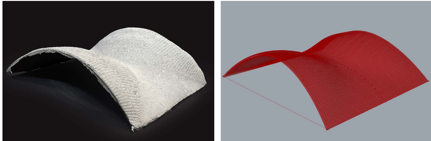
Figure 138. The 4-Quadrant (Alt Supports) pattern was 3D scanned and parametrically rebuilt as a mesh in Grasshopper. This allowed for manipulation of the edge and center curve heights as shown in Figure 139.
