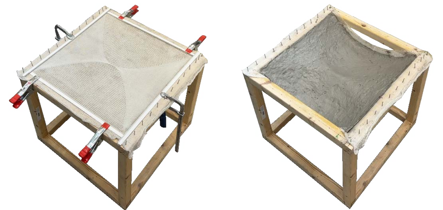
Figure 91. 4-Quadrant (Alt Supports) pattern before casting (left) and after casting (right). A 500x500 casting frame was used for the pattern combination tests and followed the same methodology described in Section 4.1.
