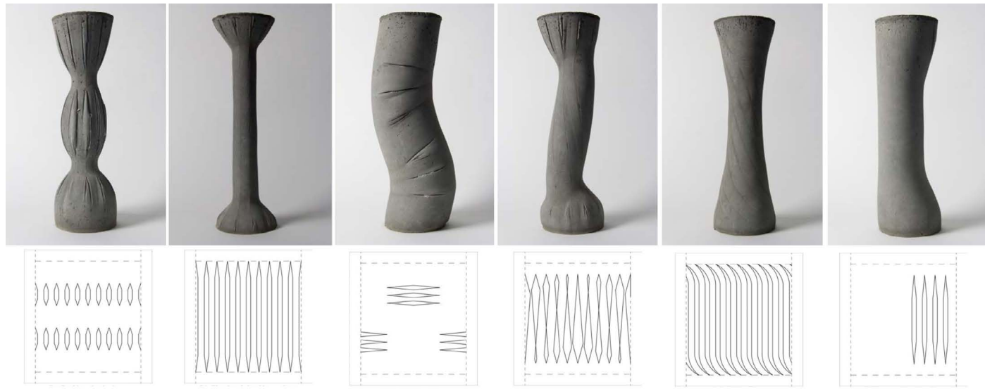
Figure 20. Six dart columns with corresponding tailored fabric formwork patterns (Milne et al., 2015)
