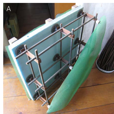
Figure 27. (A) Structurally Insulated panel with incorporated flexible formwork (B) Various residential projects in Japan with flexibly formed concrete walls (Source (all): Kenzo Unno)
