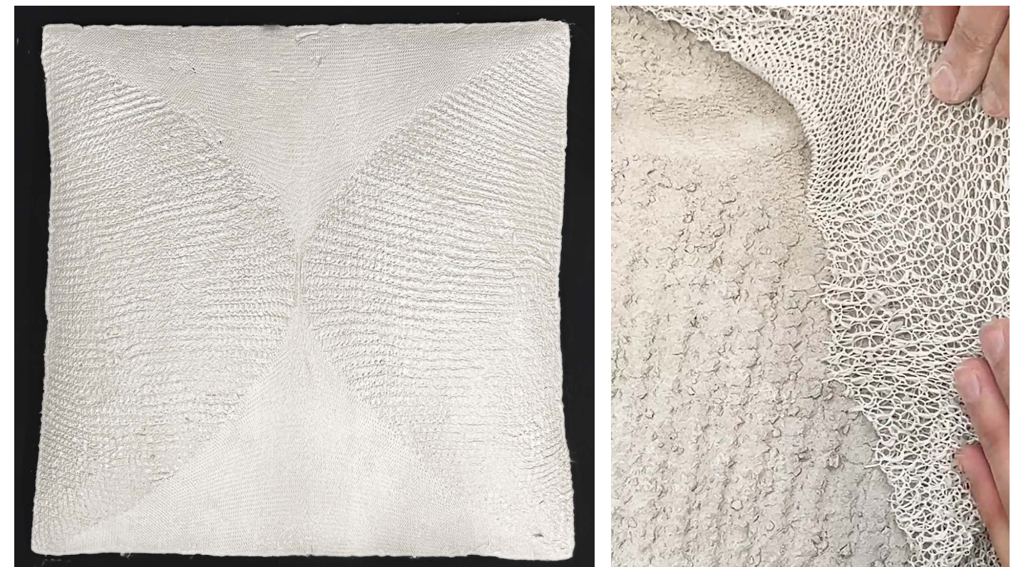
Figure 96. (Left) Top view of 4-Quadrant casting result after removal of textile, (Right) Removing the combination pattern textile.
