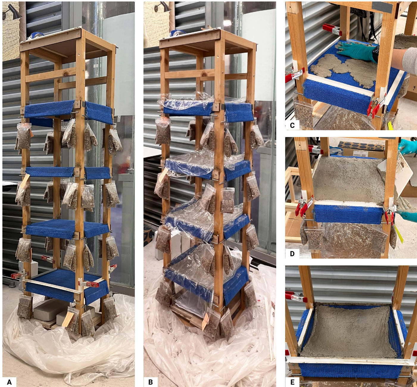
Figure 62. (A) Casting frame prepared to receive concrete (B) Casting frame with deformed samples (C) Applying concrete directly to the textile (D) Evening the concrete to a consistent thickness with the help of plastic guides and a drywall spatula (E) Deformed sample after the supporting MDF panel is released.
