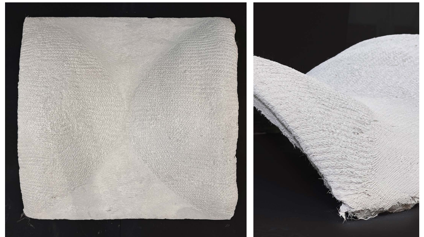
Figure 102. (Left) Plan view of 4-Quadrant (Alt Supports) casting result, (Right) Close-up view of high curvatures.
