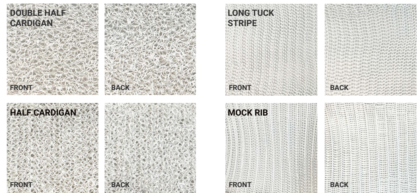
Figure 56. (Top) 2-Bed and 1-Bed tables showing the weft/warp ratios for patterns knitted with PET yarn. (Middle) 2-Bed and 1-Bed tables showing the total stitch magnitude for patterns knitted with PET yarn. (Bottom Left) Close-Up images of 2-Bed patterns with the smallest (Double Half Cardigan) and largest (Half Cardigan) total stitch magnitude knitted in PET yarn. (Bottom Right) Close-up images of 1-patterns with the smallest (Long Tuck Stripe) and largest (Mock Rib) total stitch magnitude knitted in PET yarn.
