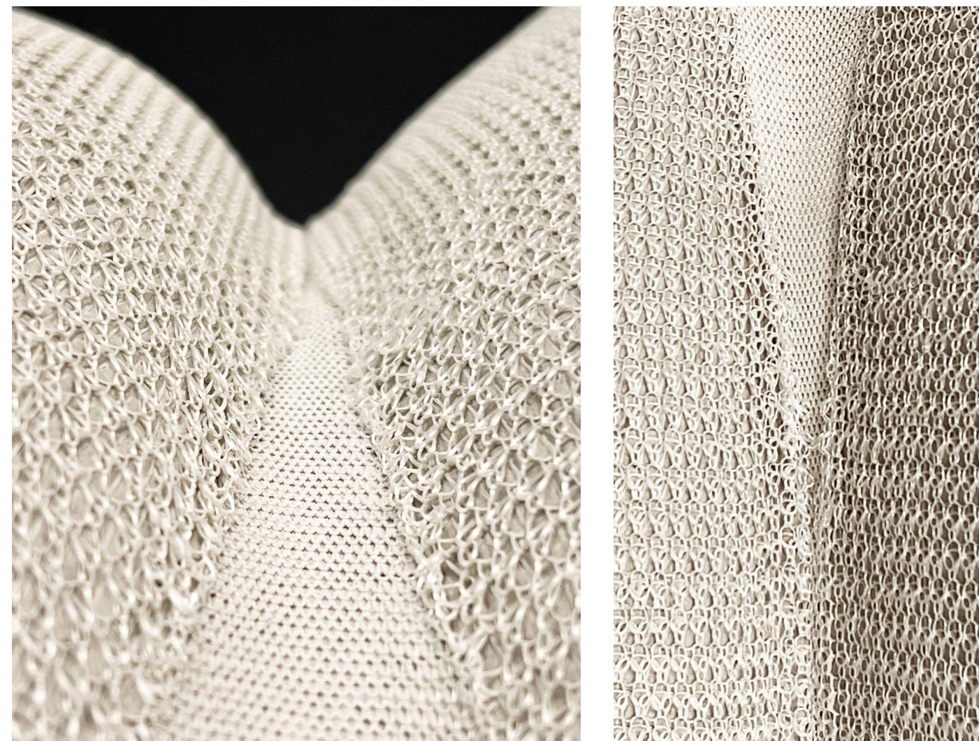
Figure 117. Close-up images of Hourglass curvature and pattern texture.
