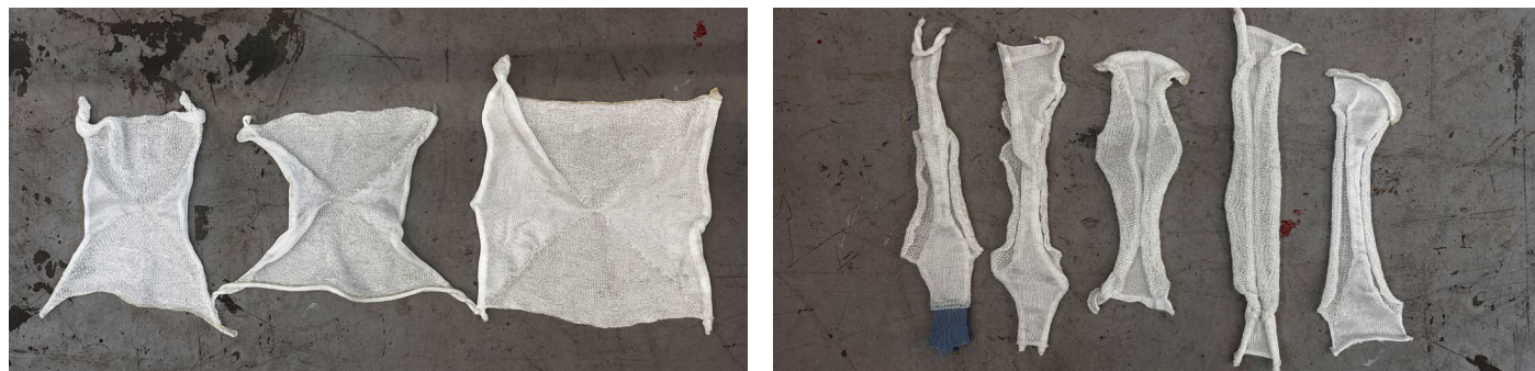
Figure 135. (Left) Three attempts were made to calibrate the 4-Quadrant pattern, (Right) Five attempts were made to calibrate the Hourglass pattern.
