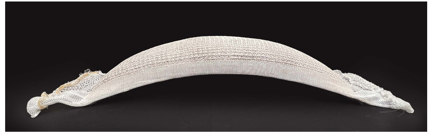
Figure 131. Side view of Half-Half casting result looking from the Cross-Miss edge.
