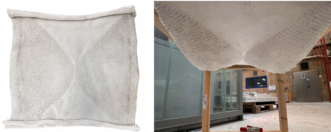
Figure 98. (Left) 4-Quadrant pattern textile after removal from the first version of this cast form, (Right) 4-Quadrant Alt-Supports on the casting frame showing high deformation at the released edges.
