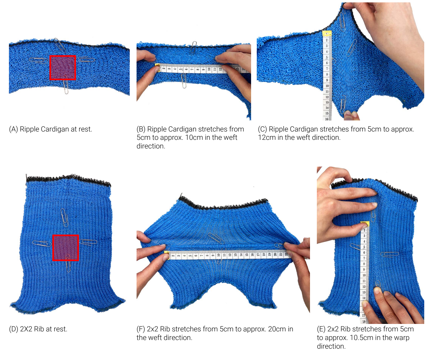
Figure 52. Of the 2-Bed pattern group, Ripple Cardigan and 2x2 Rib maintain the lowest and highest weft/warp ratios of 0.22 and 1.25 respectively. In these images, both textiles were stretched to their perceived maximum point in the weft and warp direction within a 5x5cm area marked by pins. It is evident that Ripple Cardigan stretches more in the warp direction than in the weft, and 2x2 Rib stretches more in the weft direction than in the warp.
