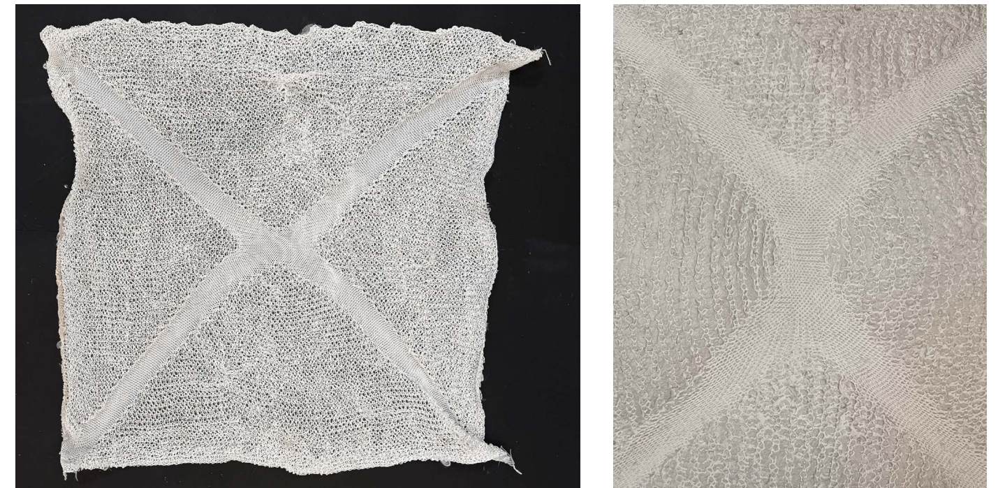
Figure 106. (Left) X-Shape pattern textile after removal showing limited damage or distortion, (Right) Close-up view of concrete texture after textile removal.
