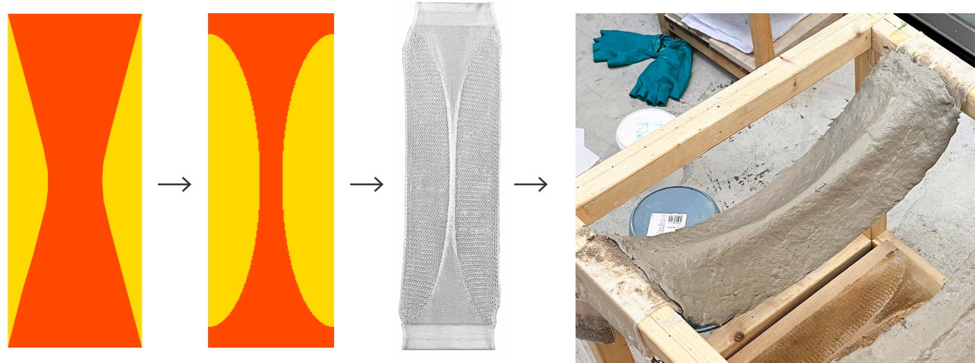
Figure 113. (Left) Desired pattern template shape, (Middle) Representation of actual bitmap pattern used to knit the sample and the finished textile, (Right) Hourglass textile immediately after casting showing extreme curvature when supported only at two ends.
