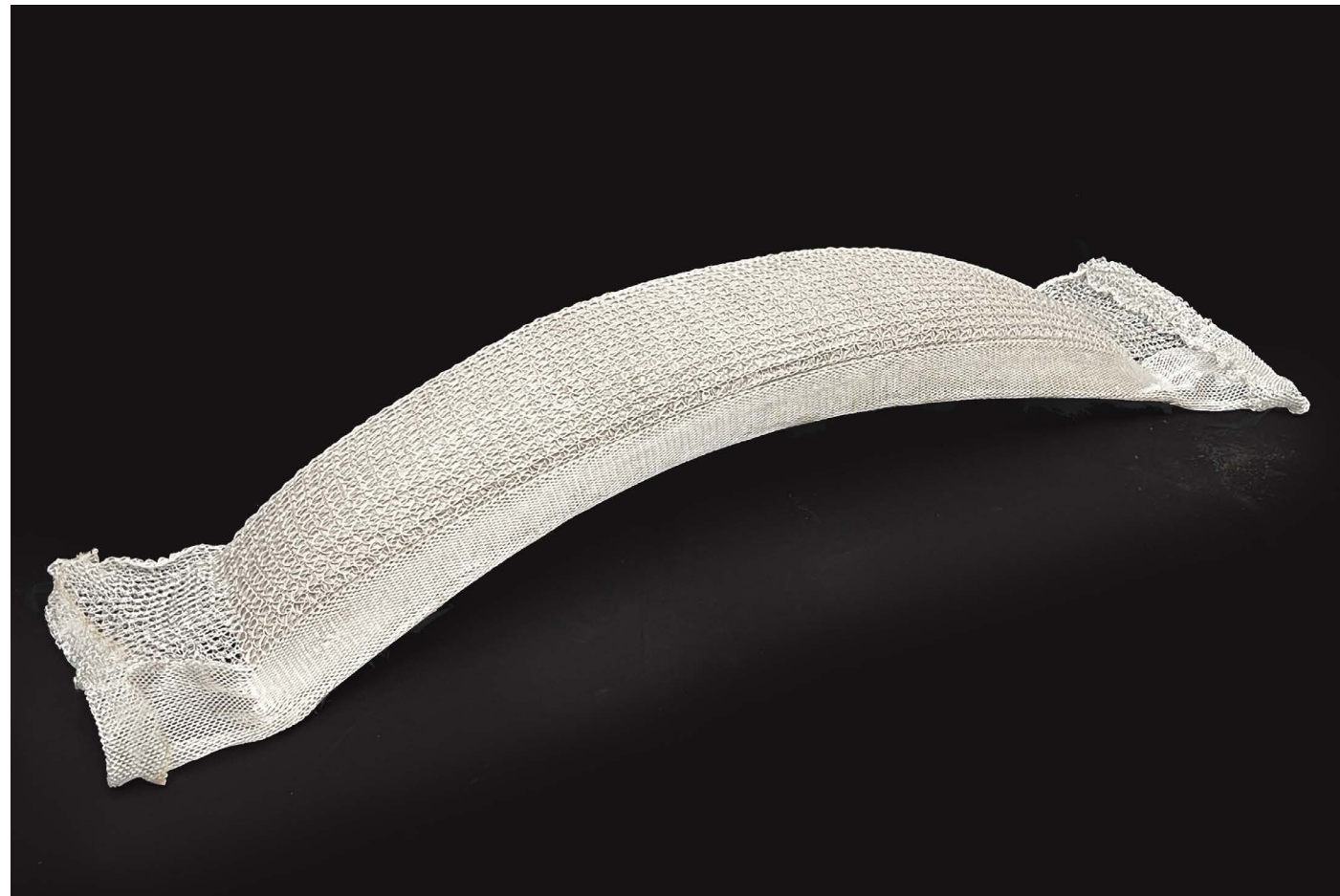
Figure 129. Perspective view of Half-Half casting result.
