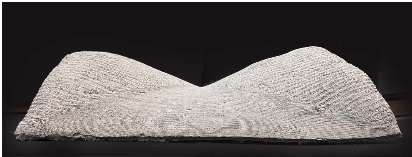
Figure 99. Side view of 4-Quadrant (Alt Supports) casting result after removal of textile.
