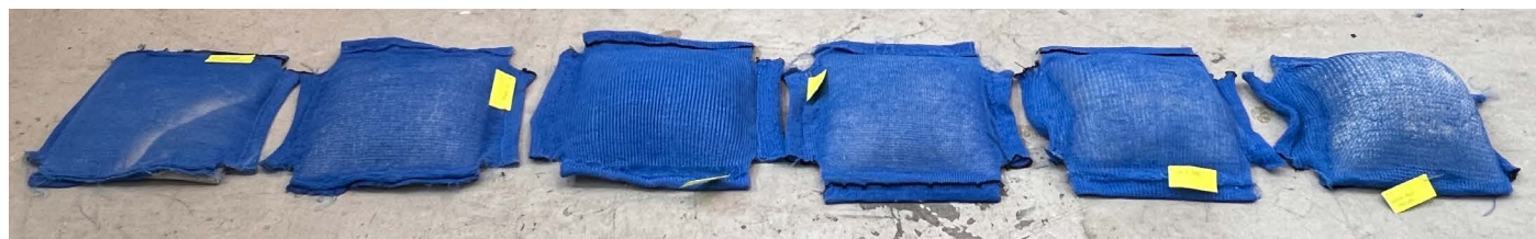
Figure 58. Group of cast samples arranged from perceived smallest to largest deformation after casting.
