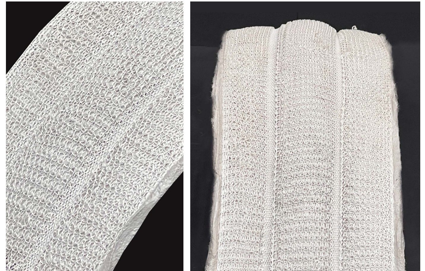
Figure 122. (Left) Close-up view of Alternating Stripe surface texture, (Right) Head-on view of Alternating Stripe casting result showing ribbed cross section with the greatest deformation at the center rib.
