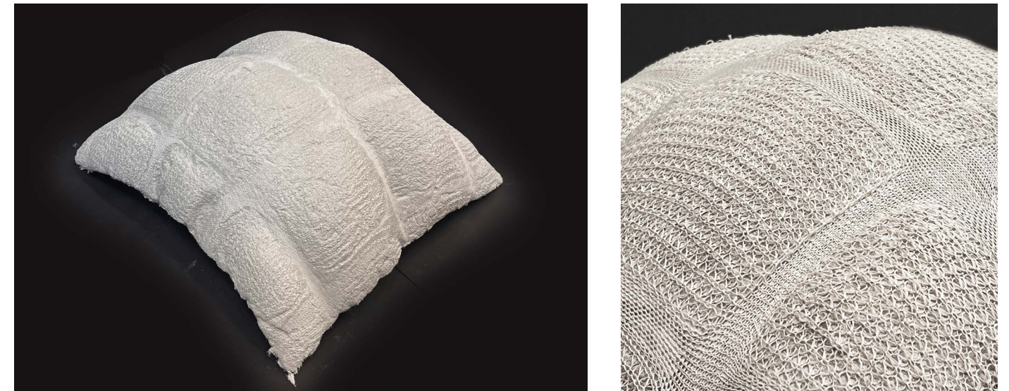
Figure 111. (Left) Perspective view of Grid casting result after textile removal, (Right) Close-up view of Grid pattern texture.
