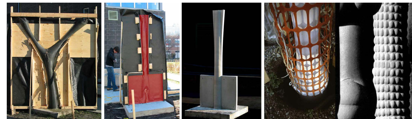
Figure 19. Various flexibly formed columns produced by Mark West / C.A.S.T. using the bulge-wall method. (Source (all): Mark West / C.A.S.T.)
