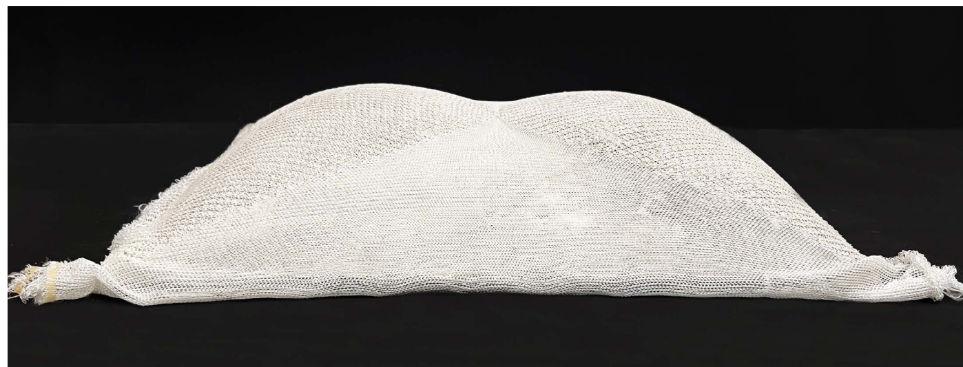
Figure 93. Side view of 4-Quadrant casting result after removal from frame.
