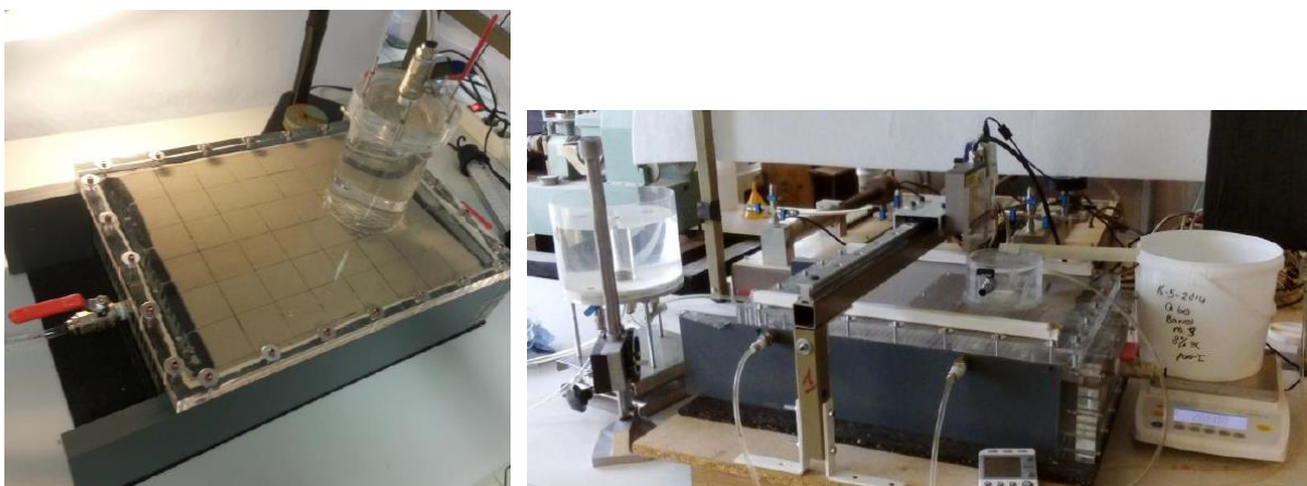
Figure 2.19: Top view of the small-scale box filled with sand (l), Overview of the full experimental set-up (r) (Vandenoer, 2018).
