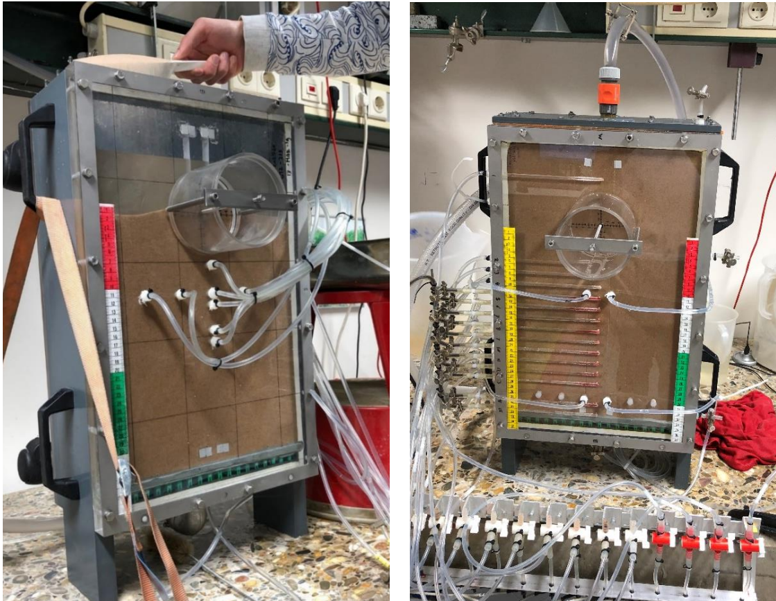
Figure 3.5: Sprinkling of the sand grains into the box (l), Filled setup with the lid on top (r) (Photographed by Van Klaveren, 2019).
