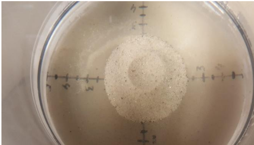
Figure 4.8: Top view of the sand boil (Outer radius = 2.1 cm).
