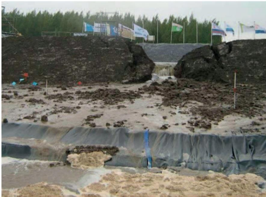
Figure 2.5: Dike breach in the IJkdijk experiments (Van Beek et al., 2011).
