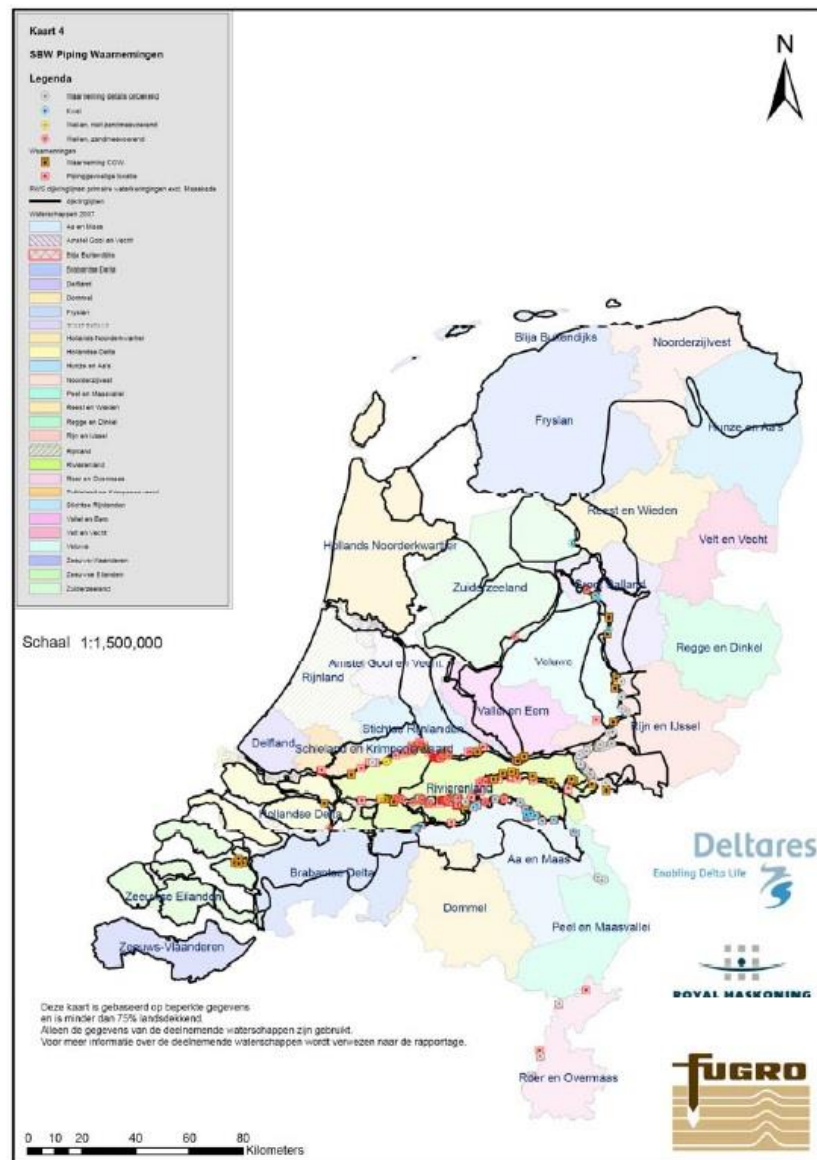
Figure 2.7: Observations of piping boils in the Netherlands (Zwang & Bos, 2009).
