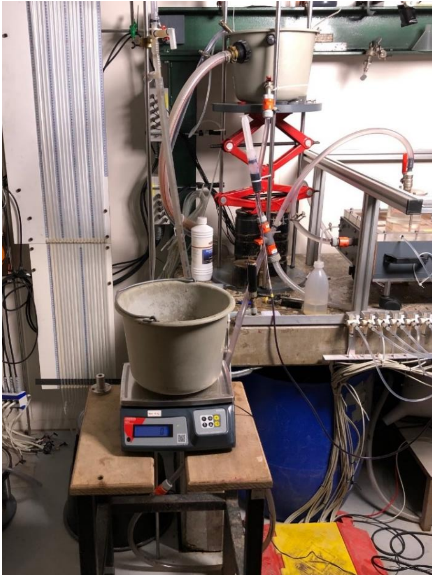
Figure 3.4: Outflow point of the experimental setup (Photographed by Van Klaveren, 2019).
