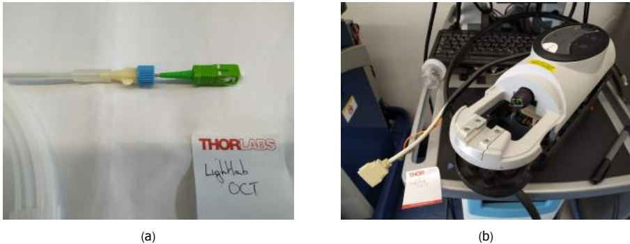
Figure A.2: Pullback system by LightLab imaging. (a) The IVOCT catheter. (b) The pullback on top of the console which controls the system.
