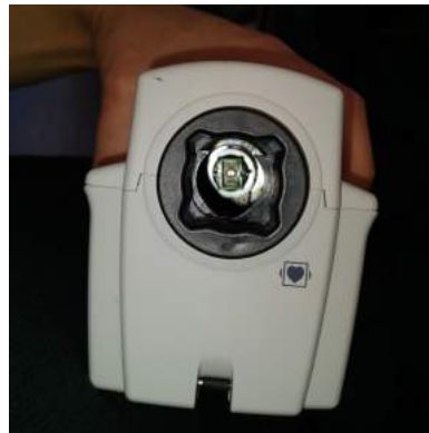
Figure A.5: Pullback system of the St. Jude Medical IVOCT Imaging system. Inside the system, mechanical alignment takes place before the optical path is fully connected.
