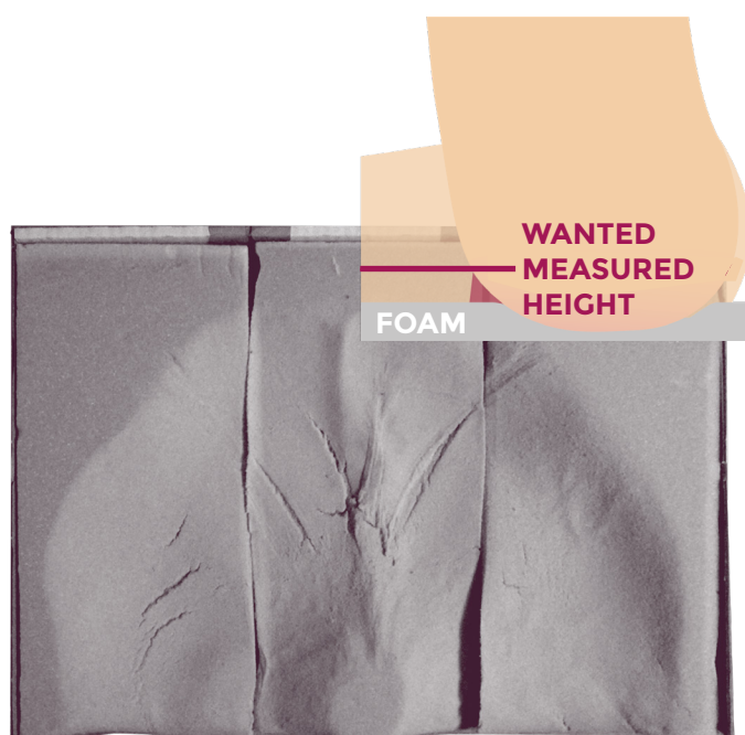
Figure 33 The result of the foam imprint test, where the foam was not thick enough to capture to full shape
