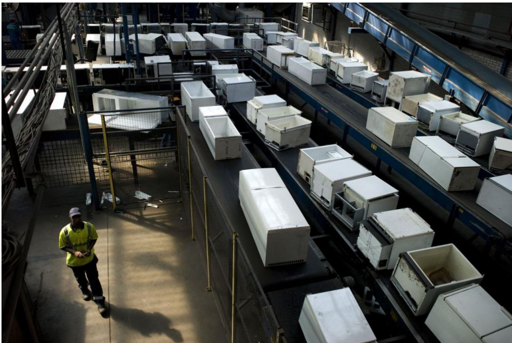
Figure 18: fridges waiting to go into the shredder after removing valuables at Coolrec in Dordrecht, NL (NRC, 2011)
