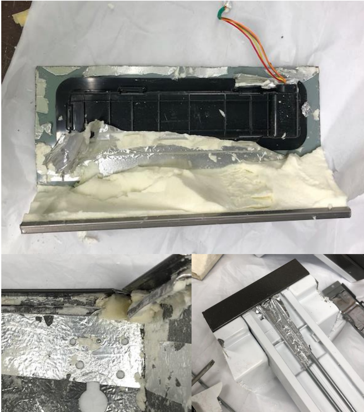
Figure 66: examples of applications of tape in the IKEA fridge (the top image doesn't show a lot of tape, but originally the whole black part was covered in tape)
