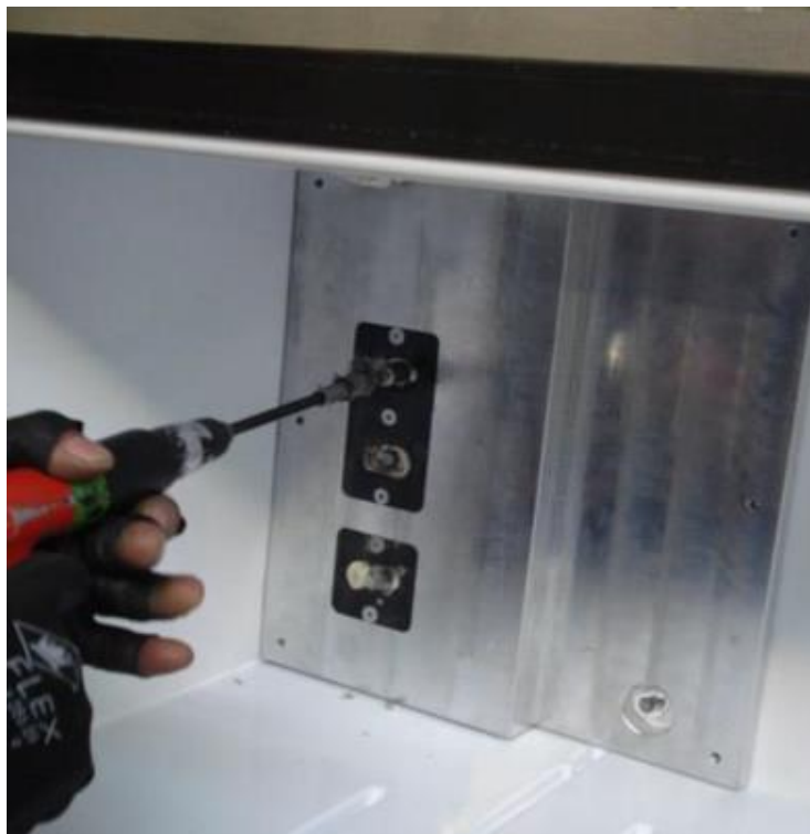
Figure 43: process plates are placed and removed because foaming doesn't allow for placement of the necessary part beforehand
