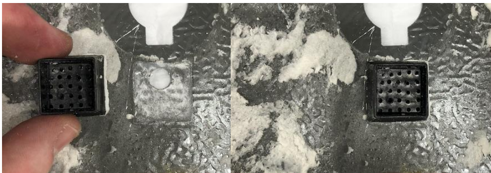
Figure 61: placement of nutplate on metal wrapping
