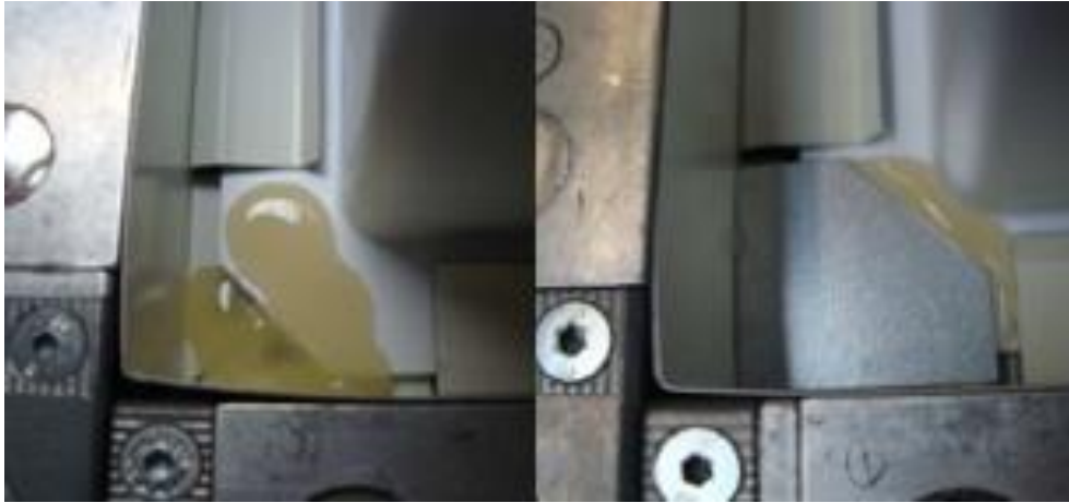
Figure 44: application of nutplate in the corner of the breaker. First hotmelt is placed then the nutplate.
