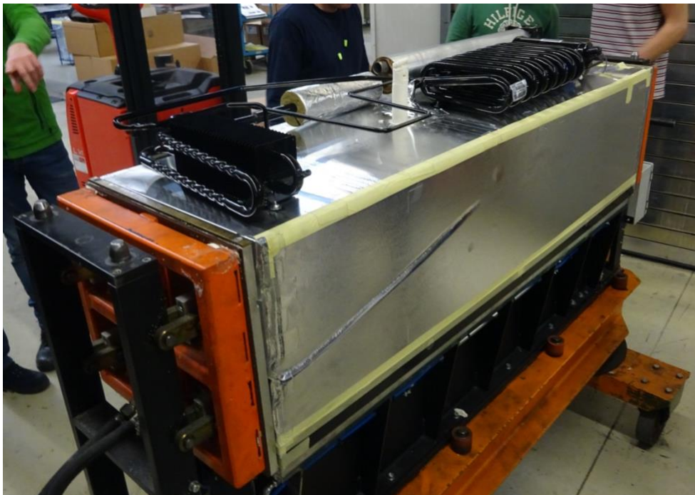
Figure 37: finished fridge after foaming
