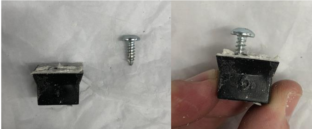
Figure 121: 'nutplate' with screw from IKEA fridge
