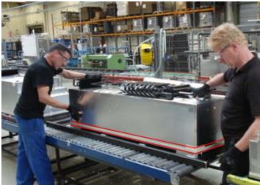
Figure 40: the wrapper is taped to the breaker to make it foam tight (masking tape is highlighted by red)
