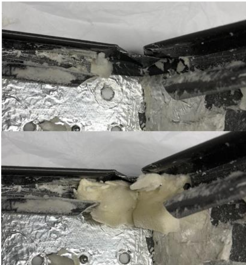
Figure 53: little piece of foam in the corner
