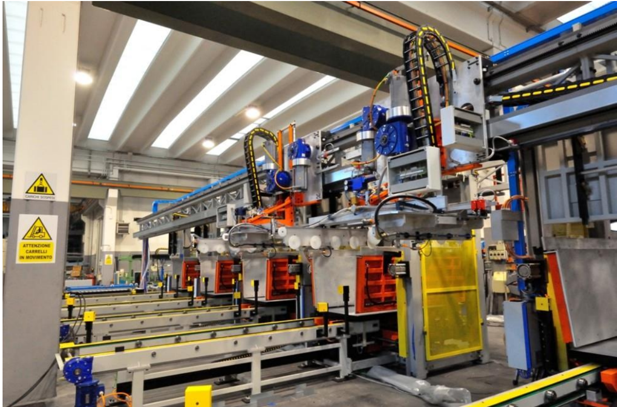
Figure 67: fully automated foaming equipment at Haier (Plastics.g, 2011)
