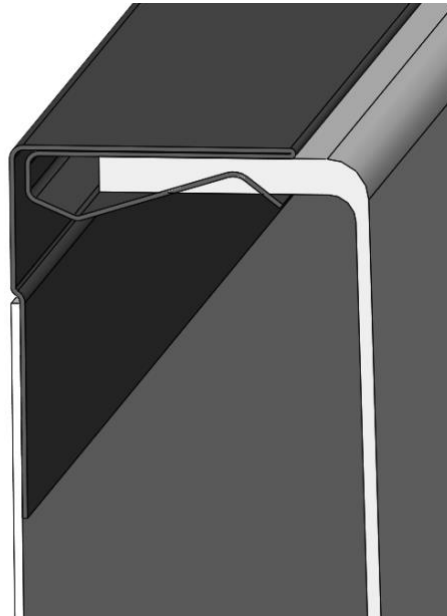
Figure 89: detail on connection breaker and wrapper concept 2
