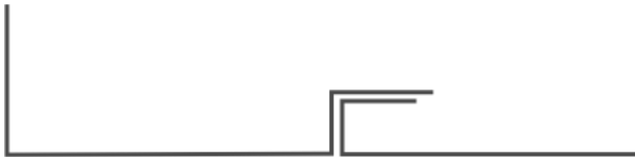
Figure 56: simplification of connection between plates
