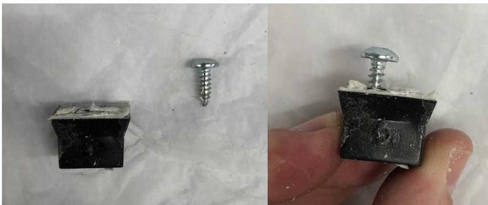
Figure 62: 'nutplate' with screw from IKEA fridge
