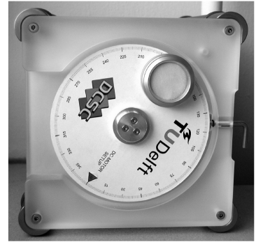
Figure 1: Schematic rotational pendulum (left), real rotational pendulum (right) 11
