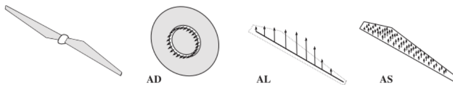
Figure 2.7: Different representations of the forces in a rotor: actuator disc, actuator line, actuator surface. From Sanderse [51].
